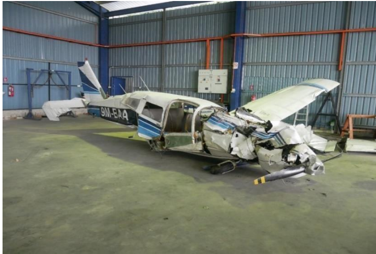
Figure 2: Aircraft condition at the hanger after salvage activities from the crash site
