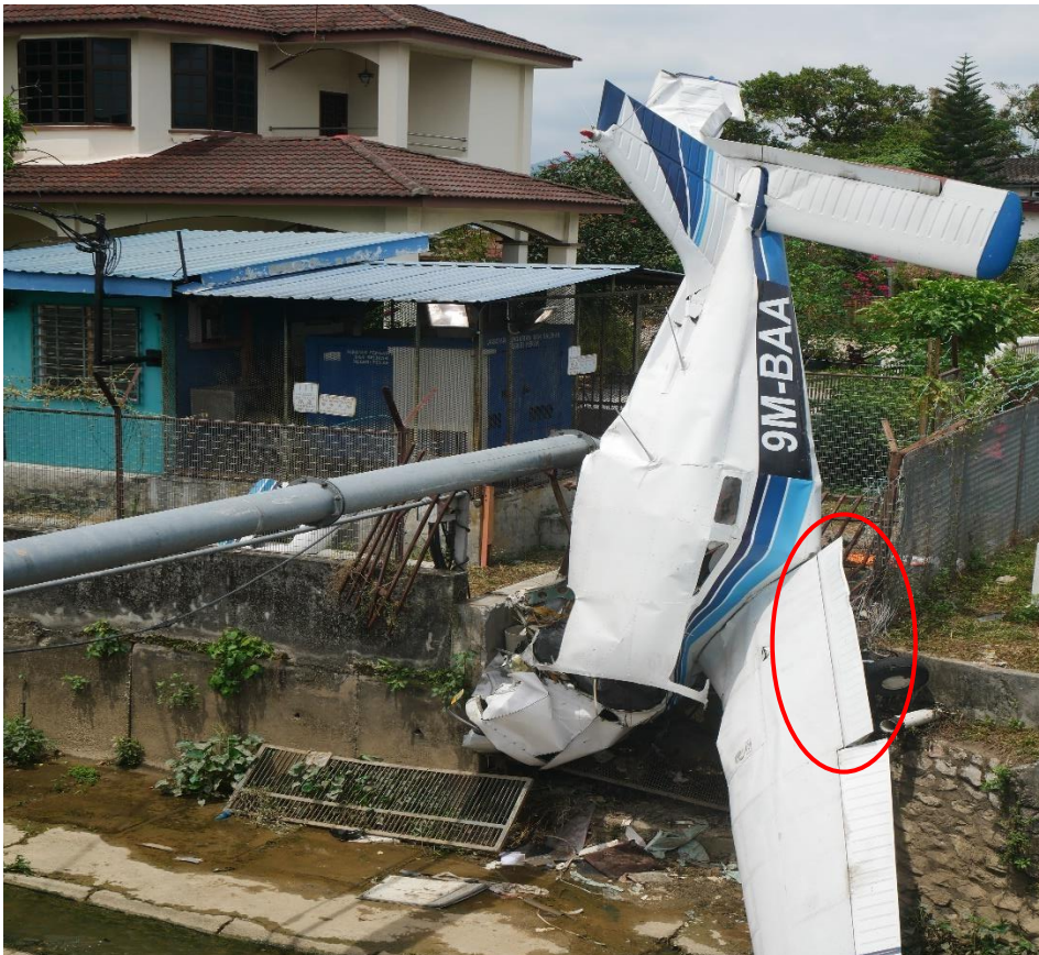
Figure 21: Flaps at UP position
