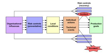
Figure 2 – ATSB adaptation of the SCM (adapted from ATSB 2008)
