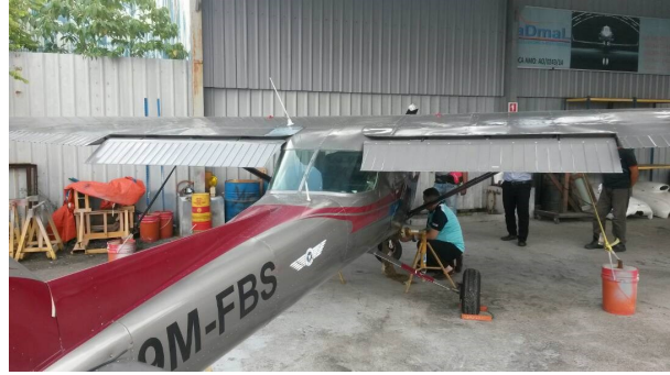
9M-FBS incident in Subang, Selangor due to hard landing and its nose wheel collapsed.
