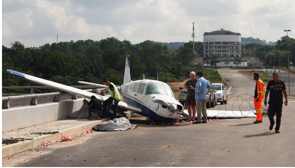
9M-DRC accident in Kulai, Johor. The accident was due to engine fuel starvation.
