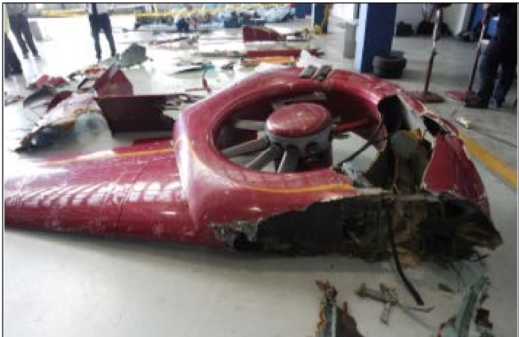
SEVERE DAMAGE ON THE LOWER PART OF THE FENESTRON
