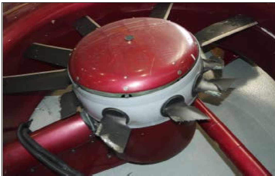
BROKEN BLADES DUE TO SUDDEN IMPACT WITH THE FENESTRON CASING
