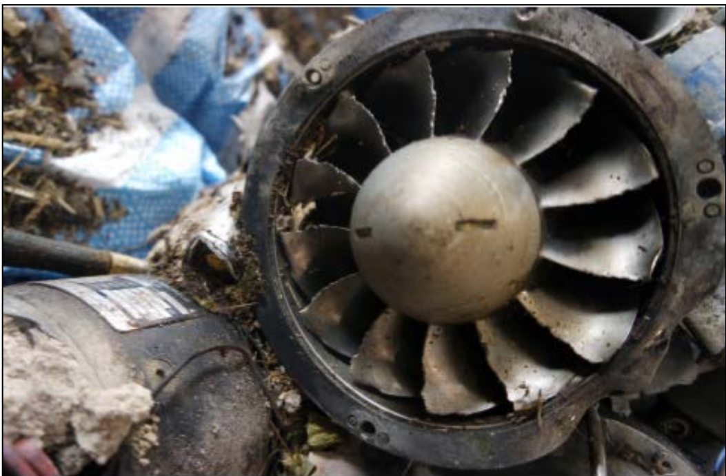
SEVELY BENT AND JAGGED COMPRESSOR BLADES DUE TO INGRESS OF FODs.
