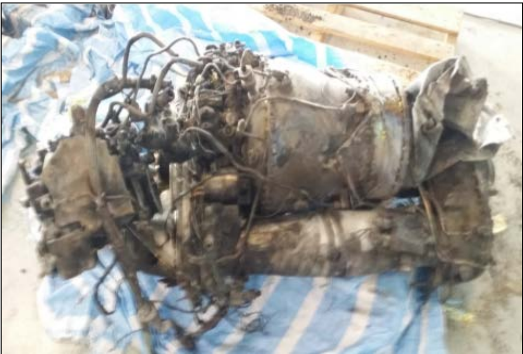
POST IMPACT FIRE ON THE ENGINE
