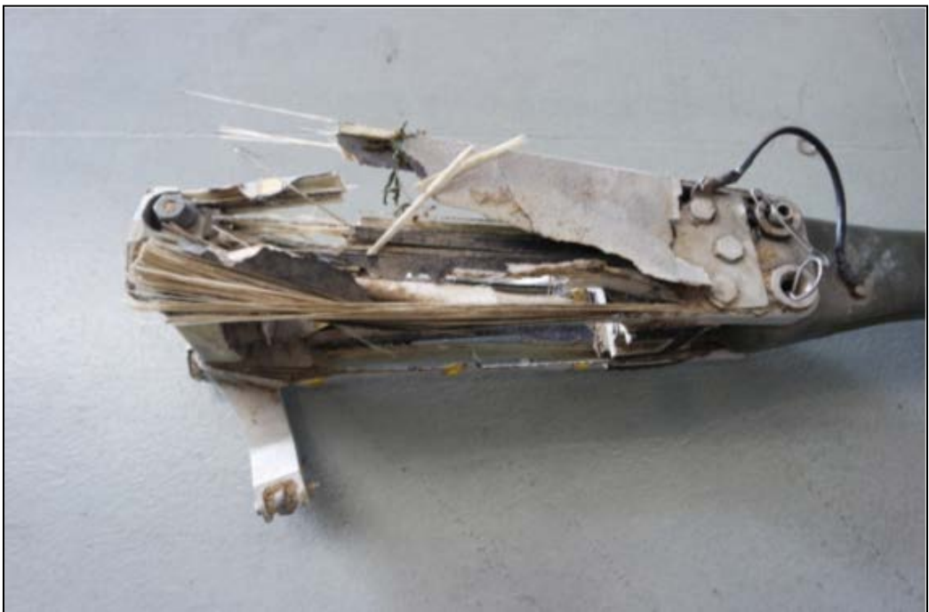
EXTENSIVE DAMAGE TO MAIN ROTOR BLADE ROOT
