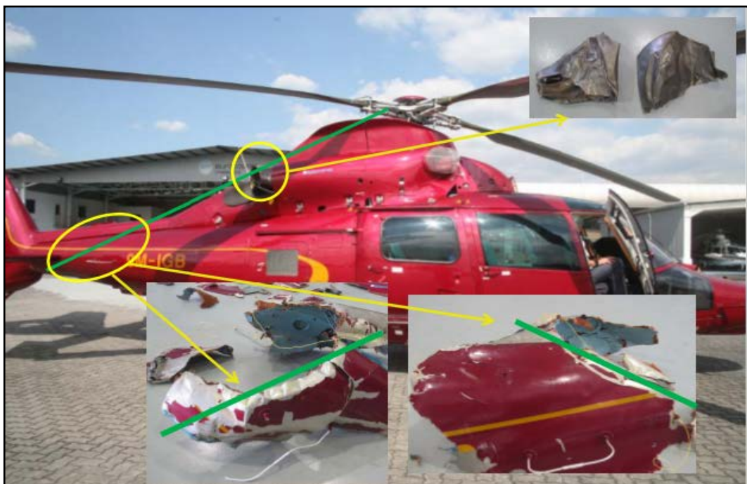
1 IMPACT EVIDENCE ON THE TAIL BOOM(+ TAIL DRIVE SHAFT, ENGINE COWLING AND EXHAUST PIPES)
