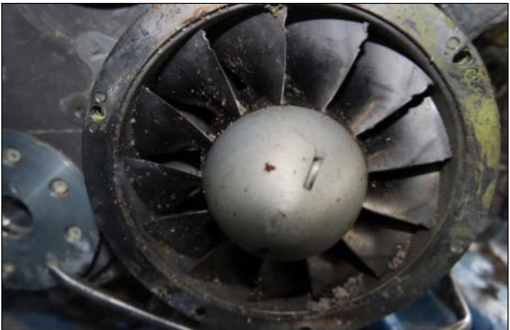
SEVERAL NICKS ON THE COMPRESSOR BLADES
