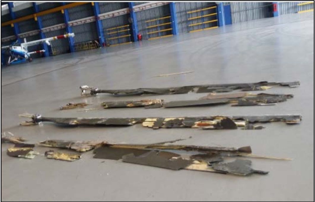
EXTENSIVE DAMAGE TO MAIN ROTOR BLADES
