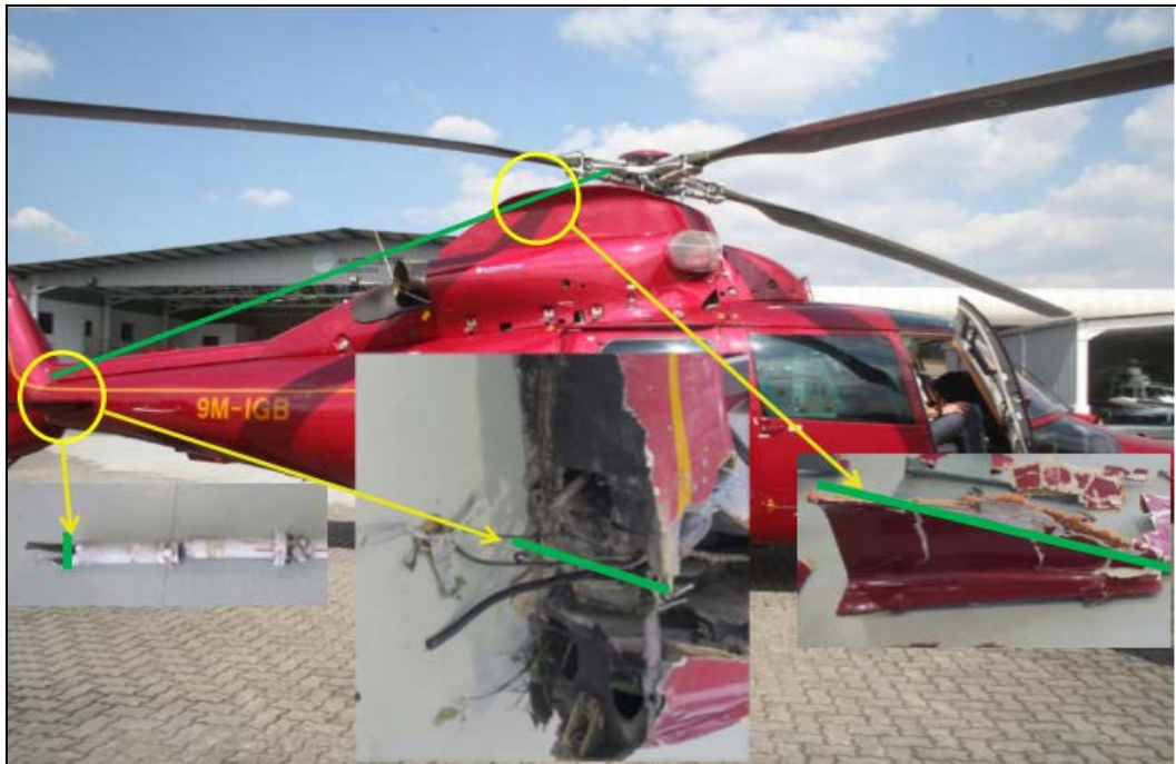
1 IMPACT ON THE FENESTRON FRAME (+ TAIL DRIVE SHAFT AND ON ENGINE COWLING)
