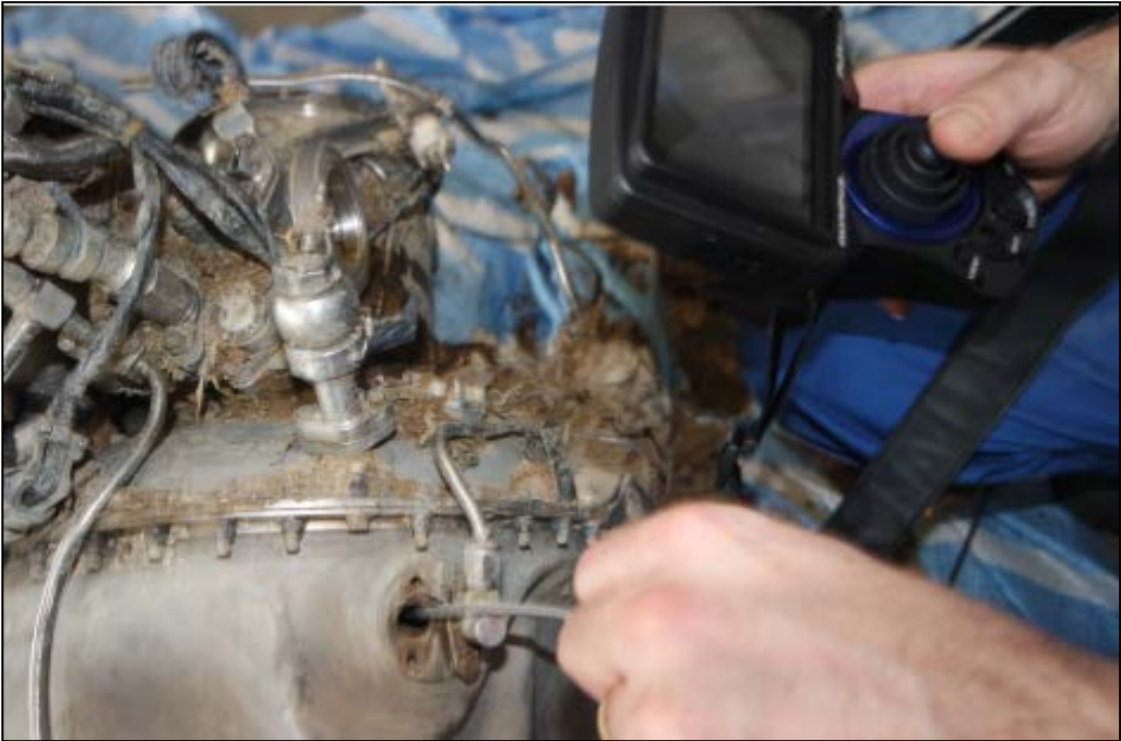
BOROSCOPE INSPECTION AROUND THE IMPELLER SECTION
