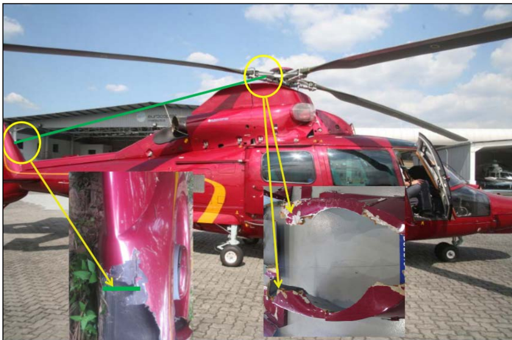
3 IMPACTS EVIDENCE ON THE REAR PART OF THE AIRFRAME
