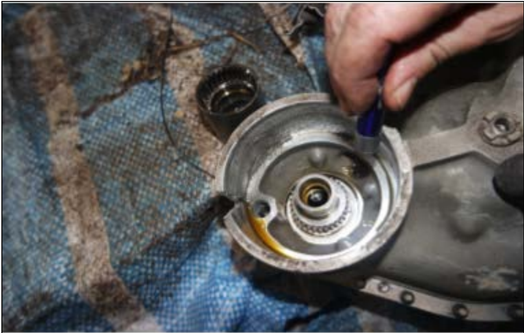
MANUFACTURER'S ALIGNMENT MARKS ON THE SPLINE AND BASE MOUNT
