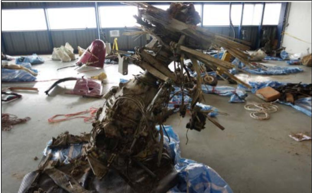
SEPERATION OF THE MAIN ROTOR BLADES UNDER HIGH ROTATIONAL SPEED
