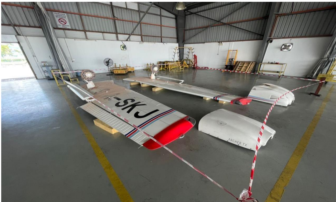
Figure 2: Aircraft condition at the hangar after salvage activities from the crash site
