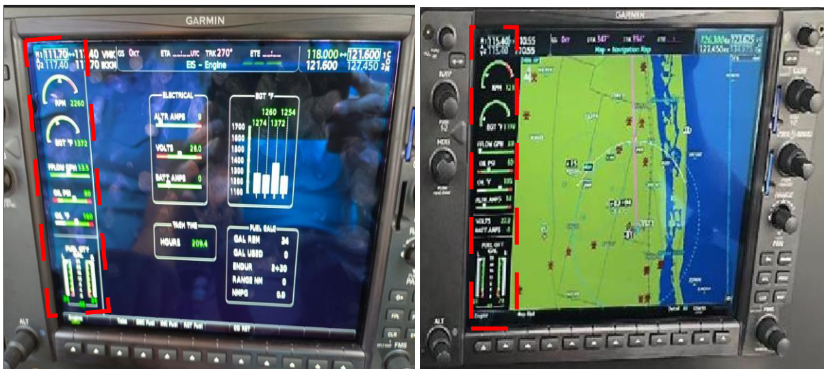
Figure 19: Engine Indicating System Page on Multi-Function Display
