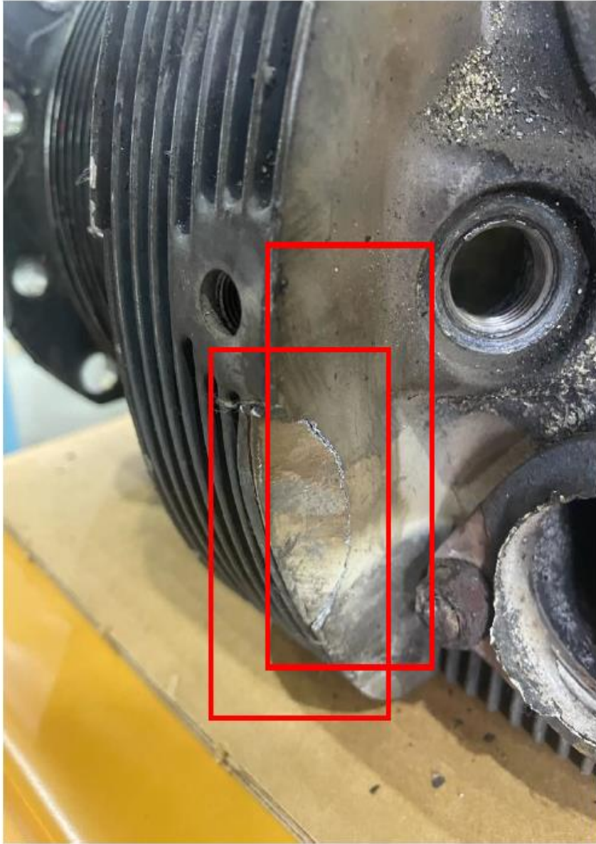
Note: Cylinder No. 1 cooling fin damage due to impact.
