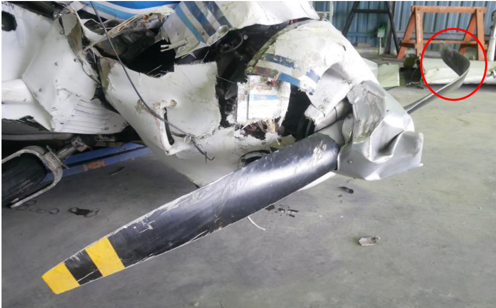
Figure 20: One propeller blade bend inwards and the other blade was in normal condition with some scratch marks
