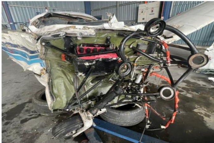
2.3.7 Engine mount broken few places
