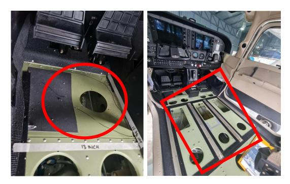
Figure 5: Forward Left and Right Floorboard Assembly found wrinkled and buckled.
