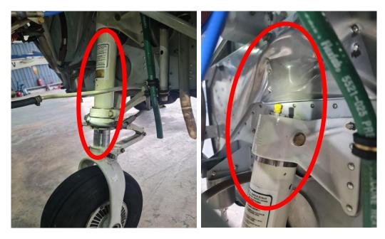
Figure 3: Nose landing gear. Damaged on riveted joints.
