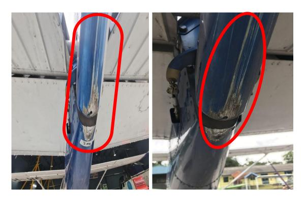
Figure 6: Rudder Lower tip found scratches
