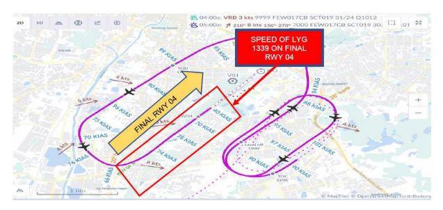
Figure 14: Data from Garmin G1000 shows the speed of the aircraft on the final to land
