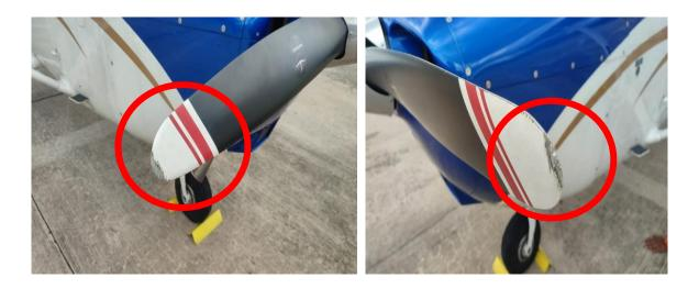
Figure 2: All Propeller blades bent inwards at the blade tips.
