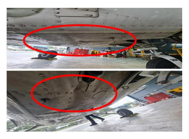
Figure 4: Below fuselage. Found deep scratches.
