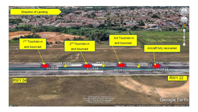
Figure 10: Landing path (Diagram not to scale)
