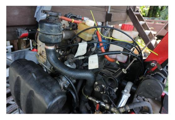
Figure 22: Removing the Throttle Cable
