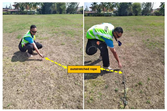
Figure 32: Outstretched rope was suspected of being stuck by the Microlight during the landing roll
