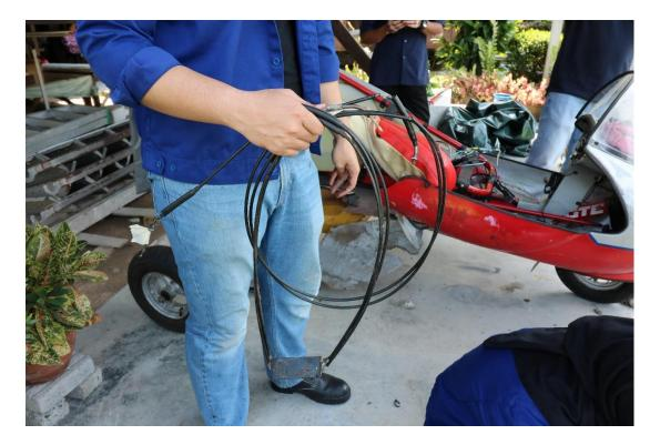
Figure 24: Removing the Throttle Cable
