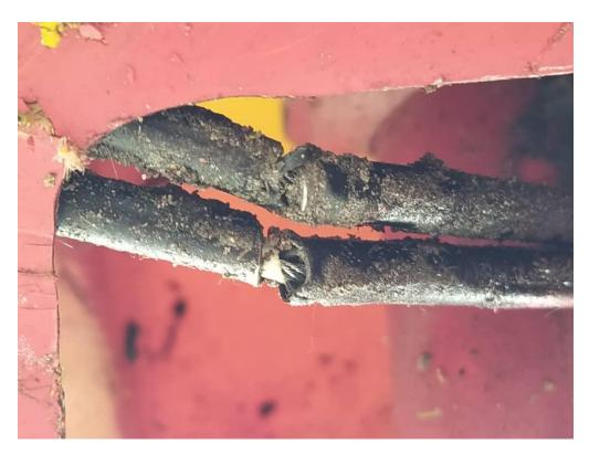
Figure 21: Post incident inspection (Throttle Cable)
