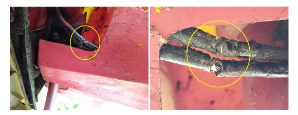
Figure 39: Post-Accident Inspection found the Throttle Cable was dented
