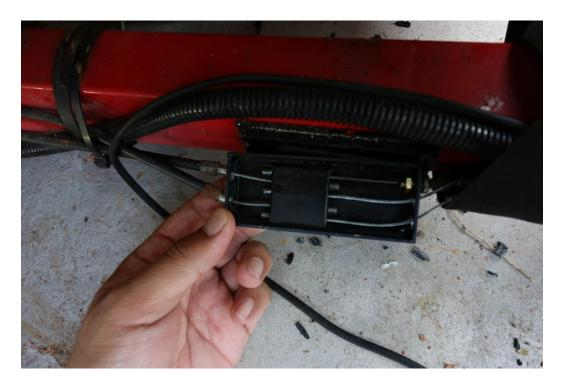
Figure 23: Removing the Throttle Cable
