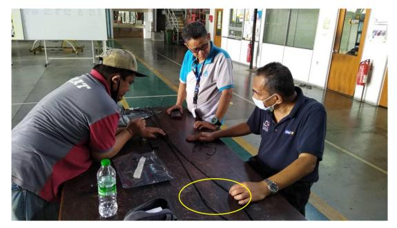
Figure 40: The Throttle Cable was sent for check and confirm that the Throttle Cable was dented
