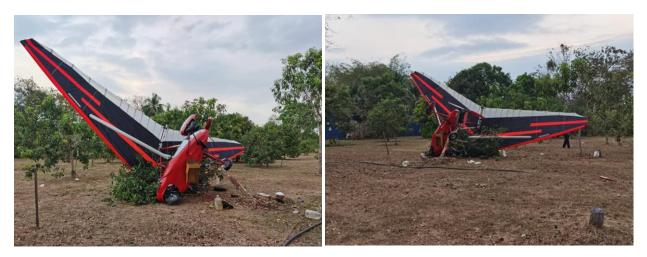
Figure 36: Microlight came to halt after hitting a small tree at the end of the landing area
