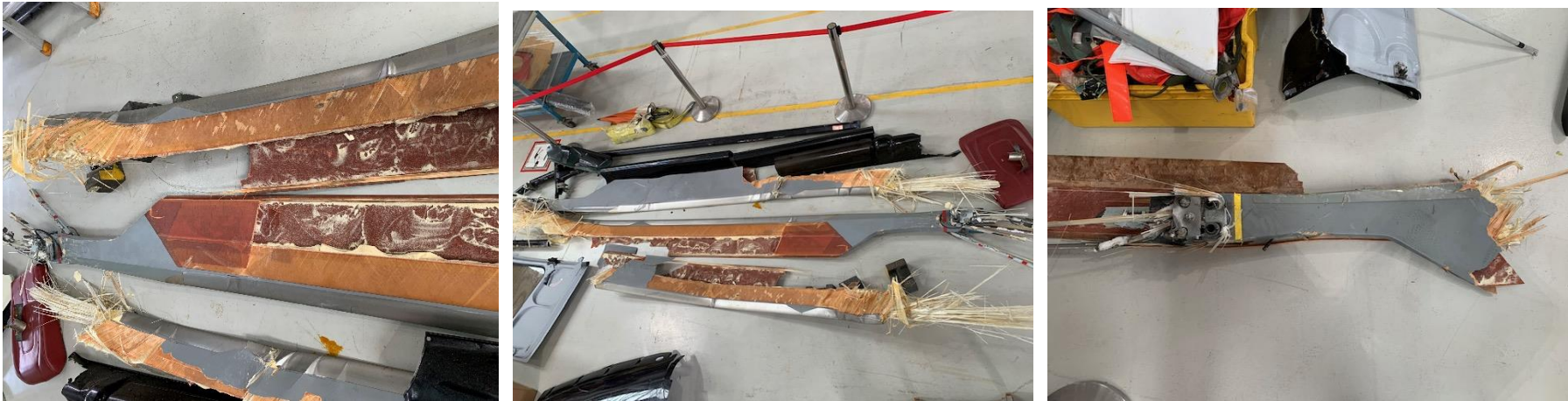
Figure 2. Damage on all the 3 Main Rotor Blades
