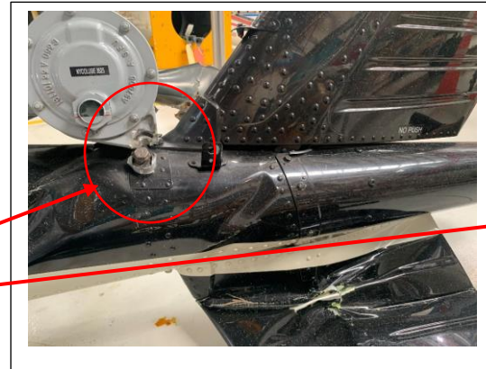
Figure 6 - Tail gear Box attachment base broken
