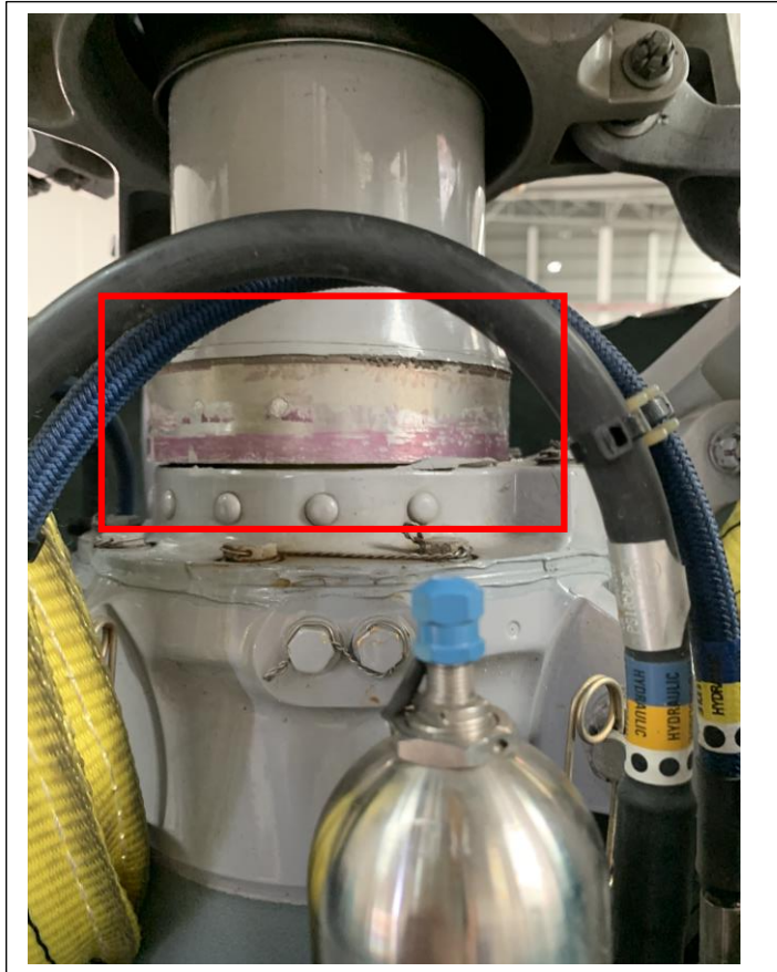
Figure 3 - Swashplate Guide – dislocated and sheared
