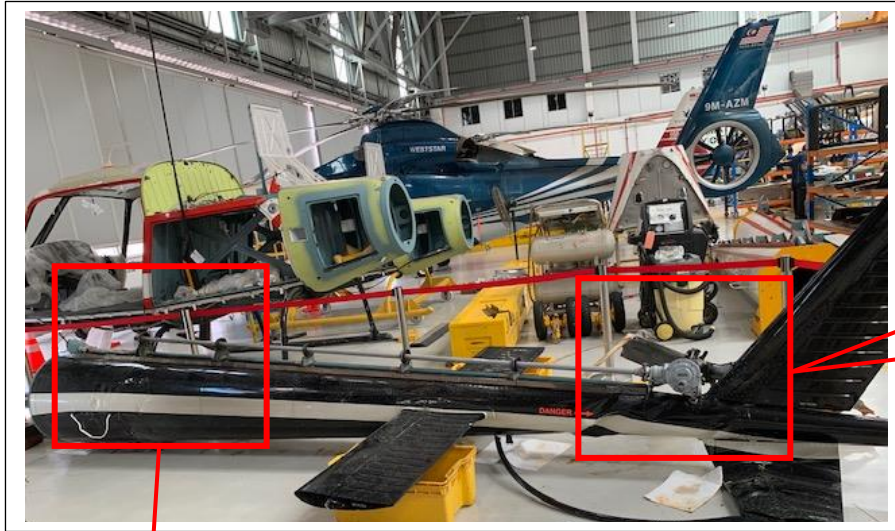
Figure 5 - Intermediate Tail Rotor Drive Shaft broken on engine side but all the attachment bolts are available
