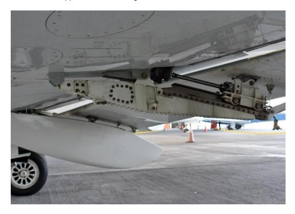
**Picture 3 –** Damages to the lower wing surface.
