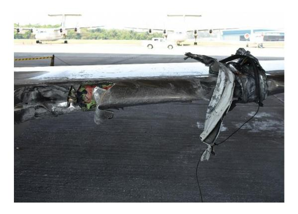
**Picture 1 –** Mid wing leading edge damages with parts of Kembara vehicle's roof stucked to it.
