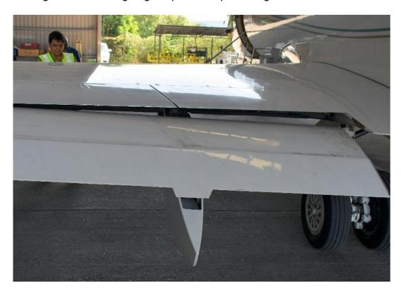
Picture 5 - Trailing edge flaps and flaps carrier
