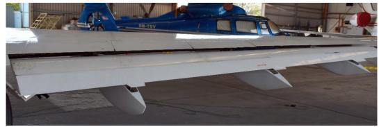
**Picture 6 -** The flaparon of the Left Wing was badly damaged as compared to the Right Wing Flaparon
