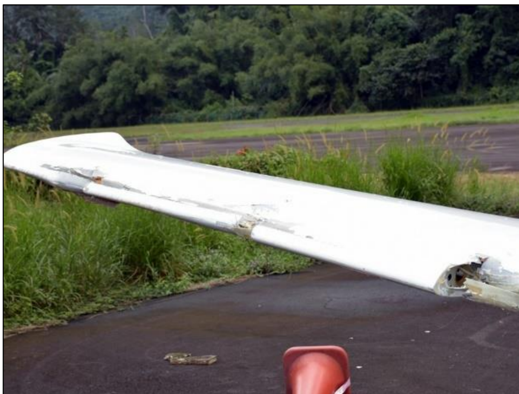
Picture 3 – Starboard side wing leading edge damaged
