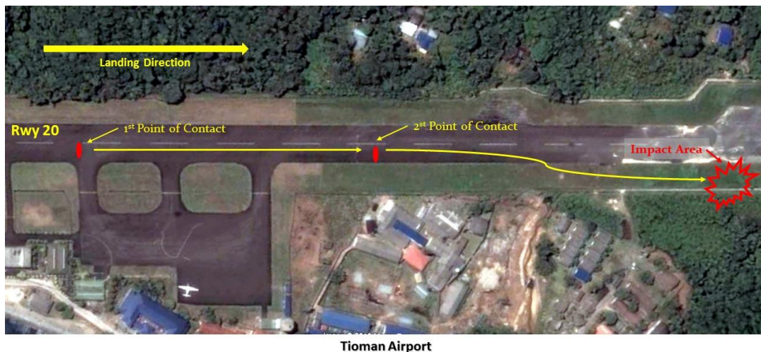
Picture 10: Illustration of the aircraft path prior impact.
