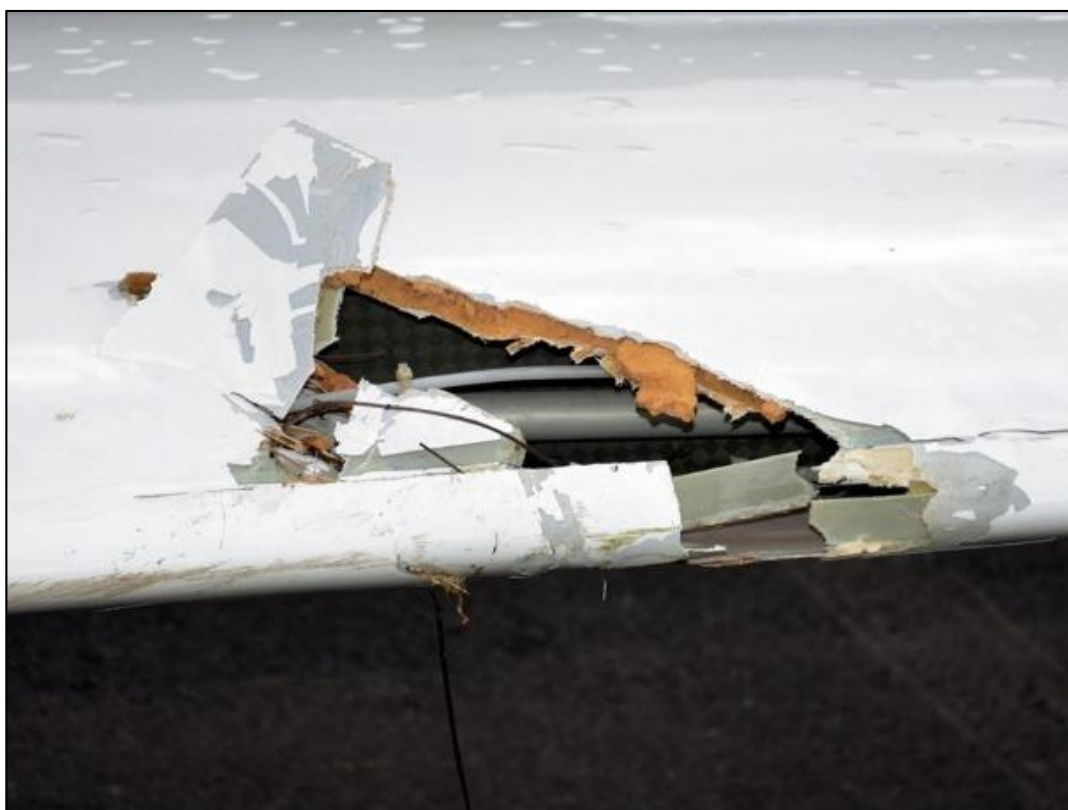
Picture 4 – Port side wing leading edge damaged
