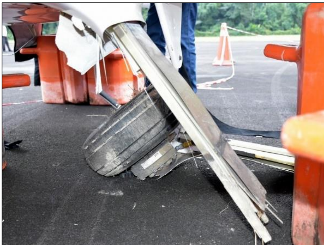
Picture 2 – Port wheel collapsed and starboard wheel damaged
