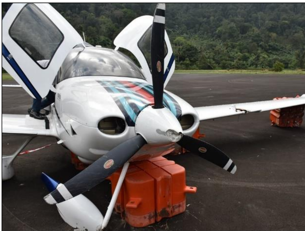
Picture 1 – Nose wheel collapsed
