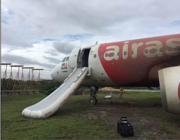
Figure 62: Aircraft Escape Slide Deployed from Door 1L
