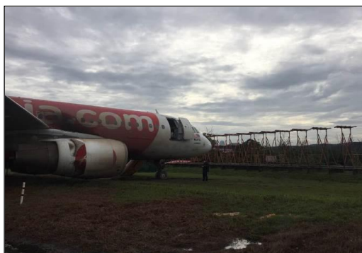
Figure 60: Aircraft Stopped 15 m from ILS Localizer Antenna Array
