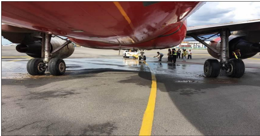
Figure 3: Long cut on LH Aft Lower Belly Fairing
