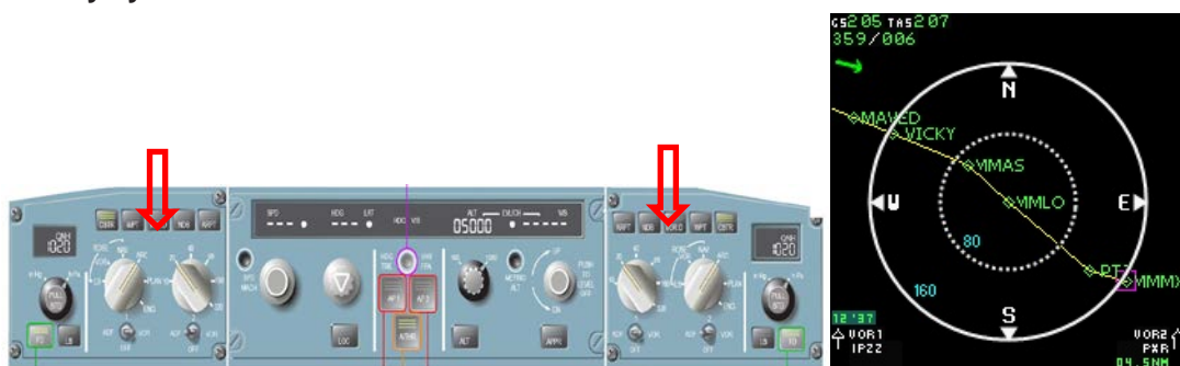
Figure 13: ND controls and an example of a PLAN mode display (right picture). Note that the track (in yellow) and waypoints (in green) are displayed but there is no aircraft or runway symbol
