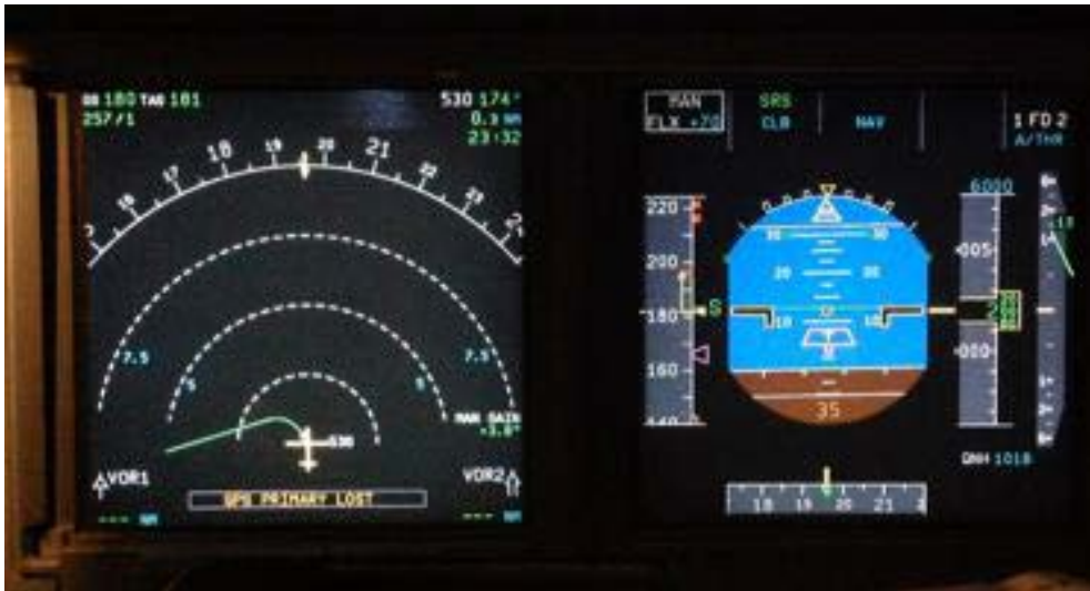
Figure 14: GPS PRIMARY LOST displayed (in amber) at the bottom-left of an exemplar ND
