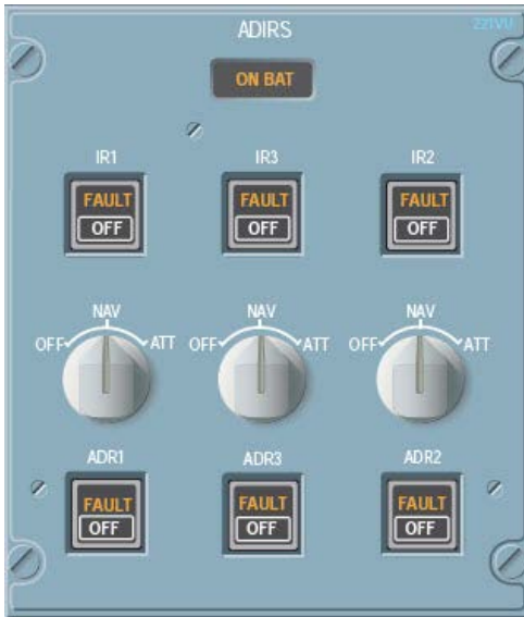
Figure 4: ADIRU rotary switches and individual inertial reference and ADR fault lights and OFF push-buttons on the A330 flight deck overhead panel
