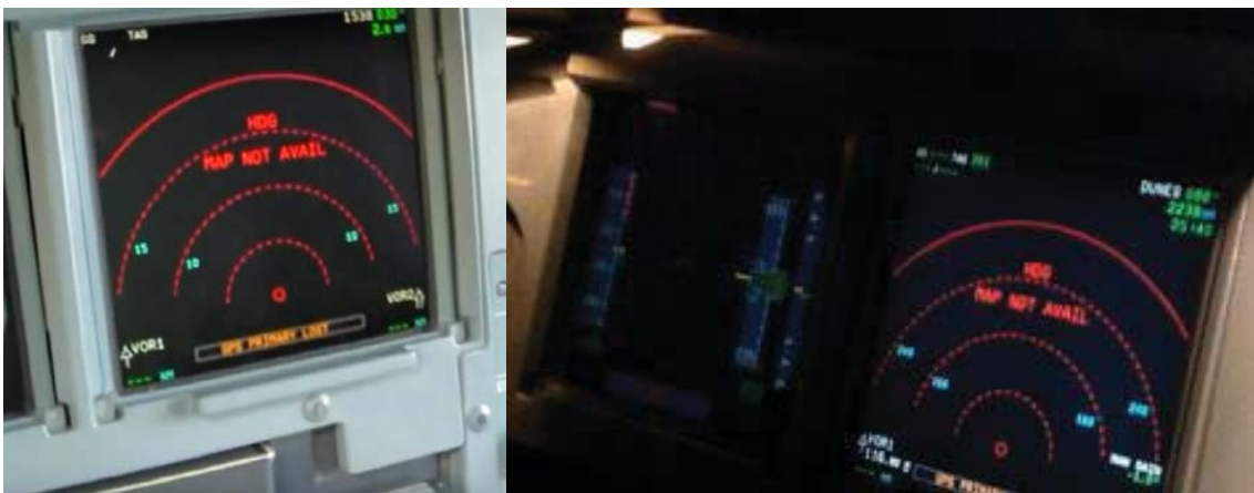
Figure 5: Simulator recreation of the captain's PFD and ND after the ADIRU 1 and 3 switches were selected off. Note the GPS PRIMARY LOST message (in amber) at the base of the photographs and the HDG and MAP NOT AVAIL message (in red) at the centre-upper of the photographs
