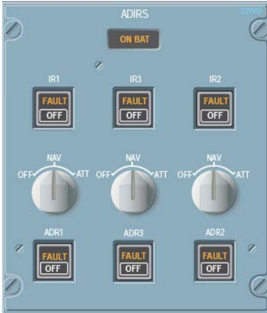
Figure 9: ADIRS control panel containing rotary switches as well as individual IR and ADR FAULT lights and OFF push-buttons.
