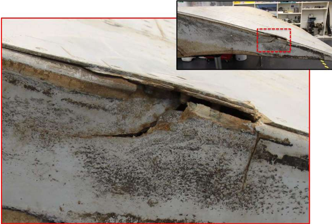
Figure 20: Outboard flap, fractured seal pan (aft)
