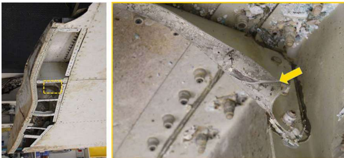
Figure 18: Outboard flap, damaged stiffeners within the seal pan cavity
