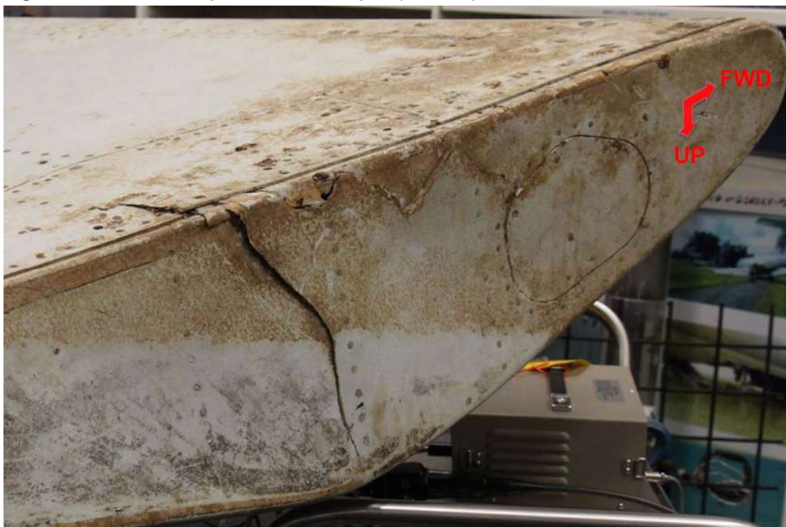
Figure 19: Outboard flap, fractured seal pan (forward)
