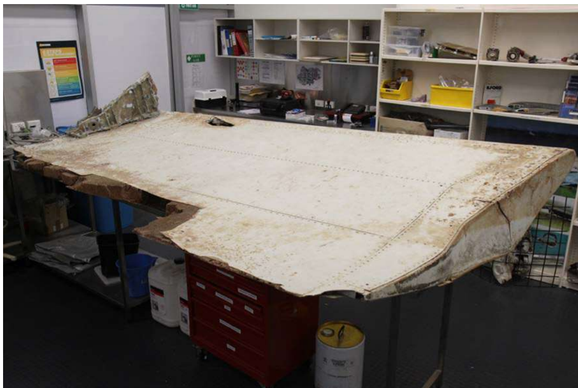
Figure 1: Inboard section of outboard flap (inverted)
