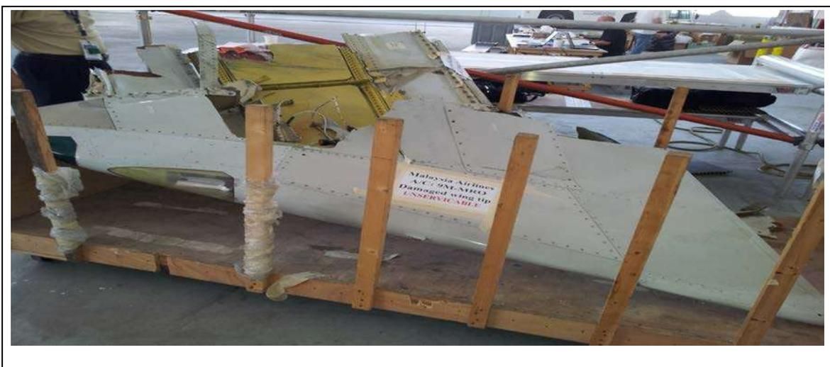
*Figure 1.6B - Damaged Wing Tip*
