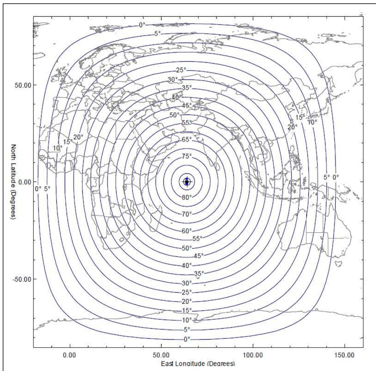
*Figure 1.9M - Inmarsat I-3 IOR Satellite Coverage Map*
