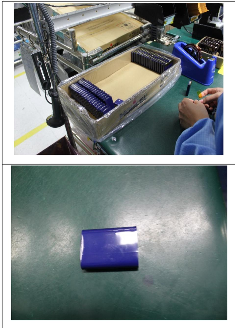
*Figure 1.18E - Raw Single Cell Battery*
