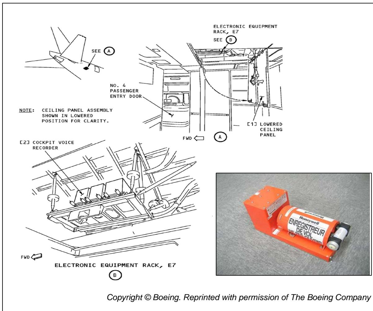
Figure 1.11B - Location of Solid State Cockpit Voice Recorder
