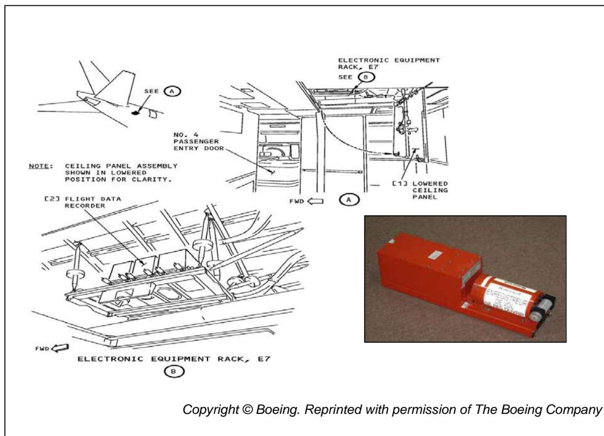
Figure 1.11A - Location of Solid State Flight Data Recorder
