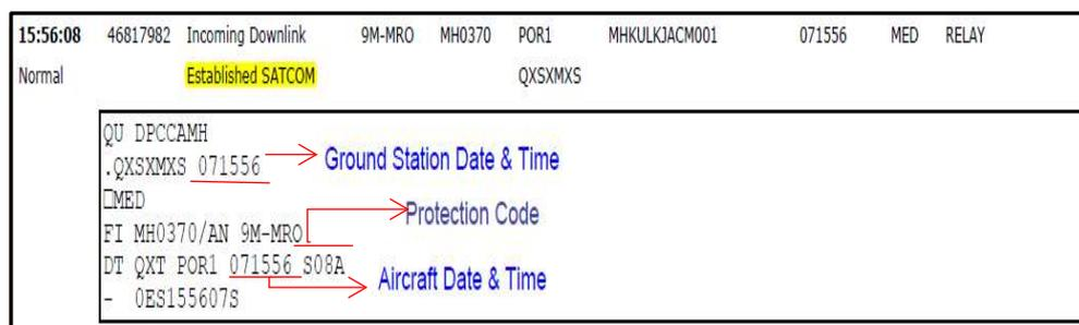
Figure 1.9C - ACARS data link established SATCOM transmission
