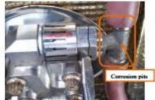
Figure 1 : Cracked B-out
