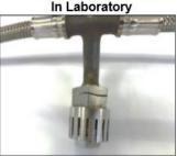
Same manifold Crack in lab. After 3 days Operator: Wings Air 22 June 2015 – Torqued at 2x EMM 25 June 2015 – cracked observed
