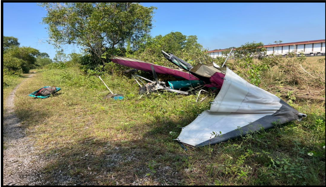
The microlight aircraft sustained significant impact damage after colliding with trees.
