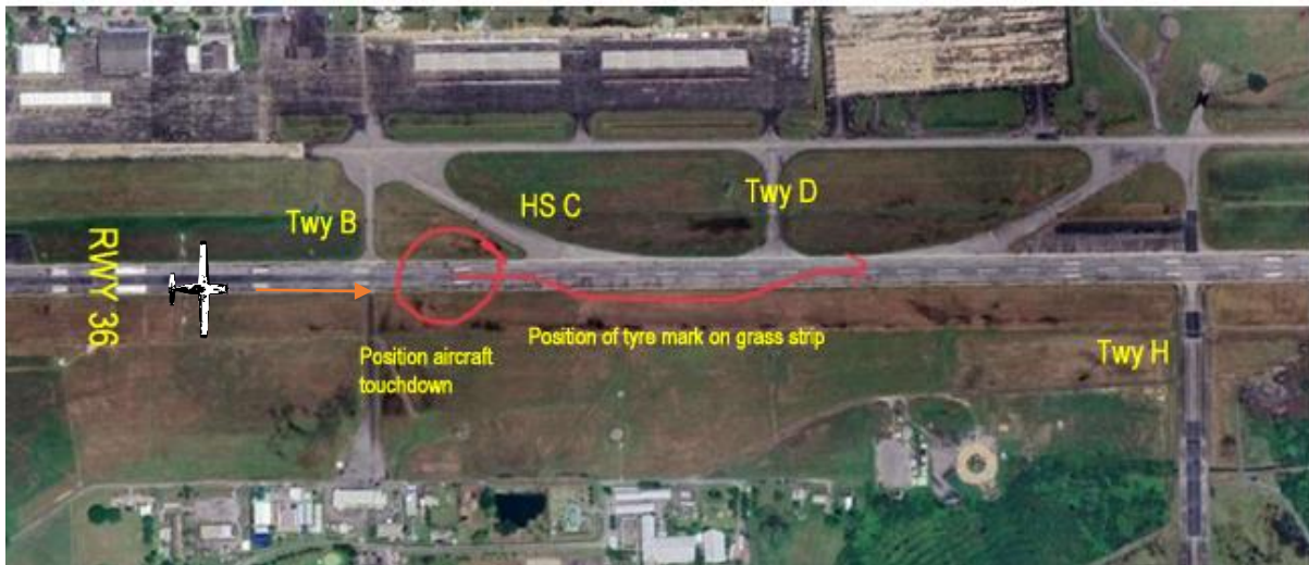
Figure 6: 9M-MXU wreckage and impact information (WMKD)
