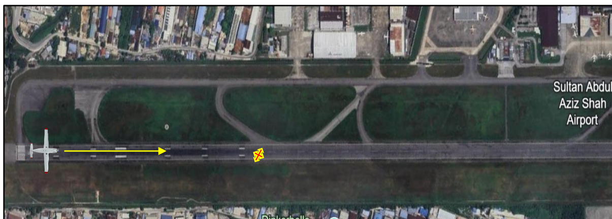
Figure 5: 9M-SKR wreckage and impact information (WMSA)
