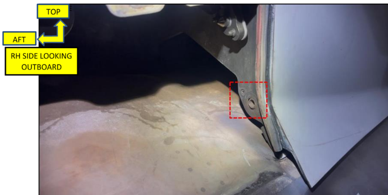
Figure 12: Loose Bearing on Engine No. 1 Pylon Inboard Panel
