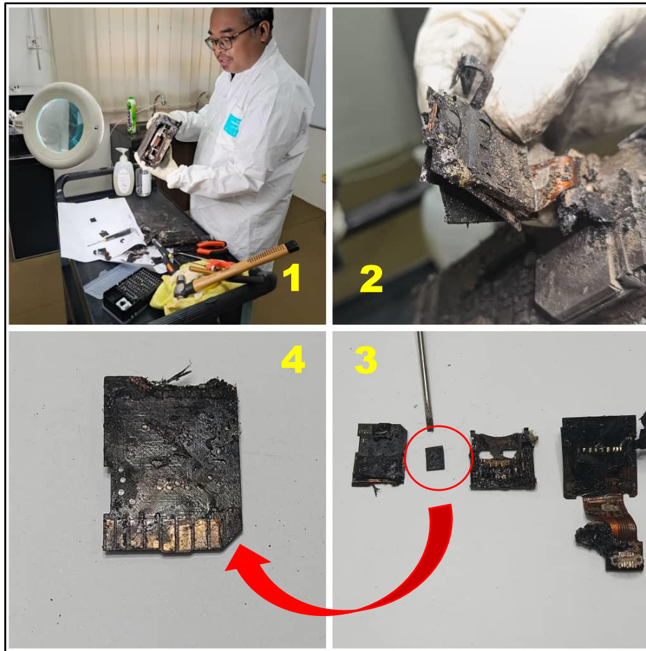
Figure 7: Retrieval of the Garmin GTN 6xx series unit memory card accessible
