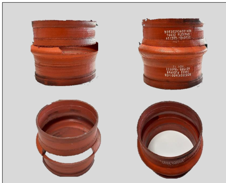
Figure 10: Condition of RH Flexible Pressure Sleeve Ruptured
