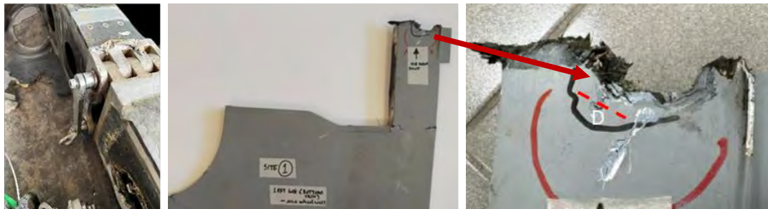
Figure 37. LH Wing – Tie-Down Ring and Man-Made Hole (Fragmented Portion)
