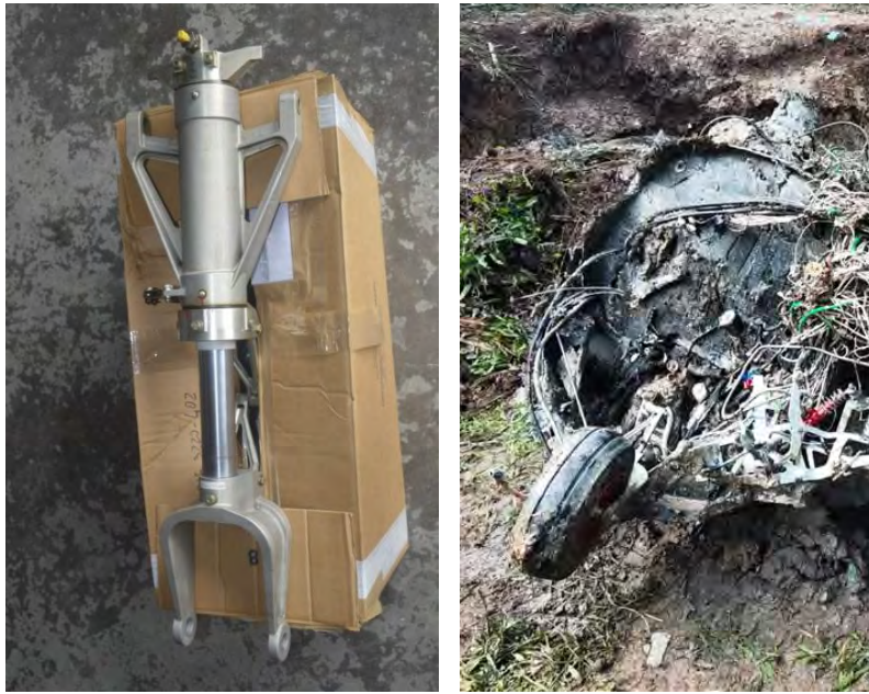
Figure 13. Old NLG Found at AAFC Hangar (Left) and Newly Installed NLG on Wreckage (Right)
