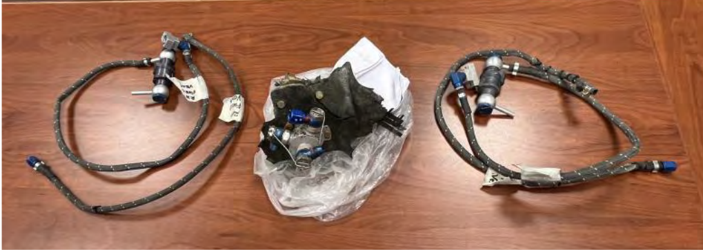
Figure 31. Fuel Components Tested by ANSV (Courtesy of ANSV) Fuel Valve (Centre); Inner and Outer Fuel Vent Lines (Left – LH; Right – RH)
