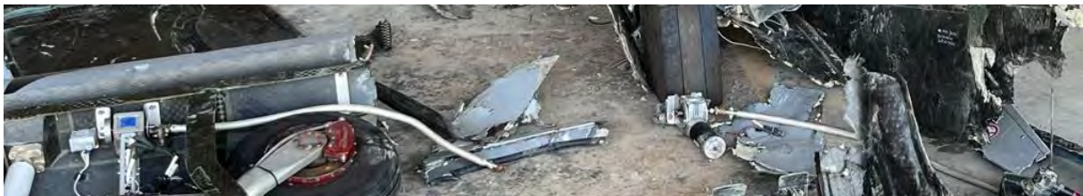
Figure 23. Flap Control System: Flap Motor and Connecting Rods
