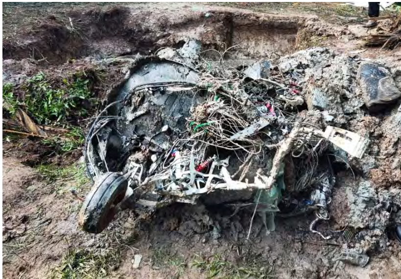
Figure 30. Nose Wheel Retracted; Impact Not Absorbed by Landing Gear.
