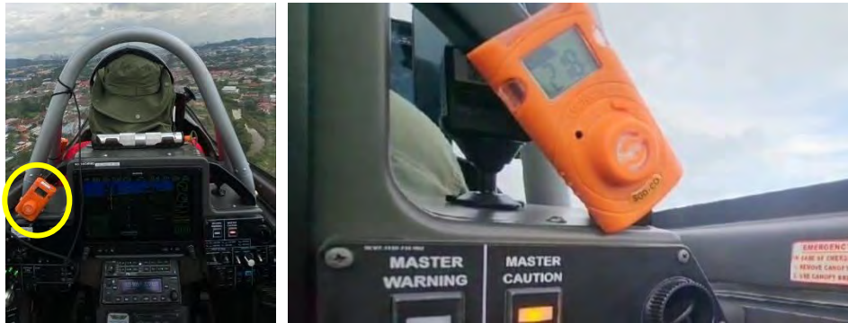
Figure 15. Jury-Rigged Portable CO Detector
