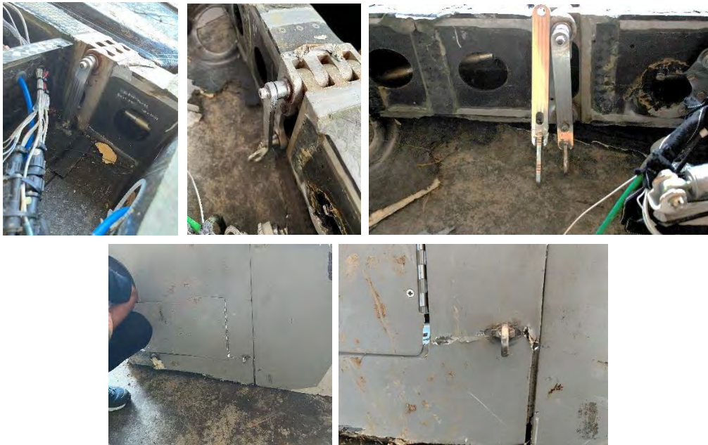
Figure 28. Non-Conforming Parts Installed on The LH And RH Wing Fitting
