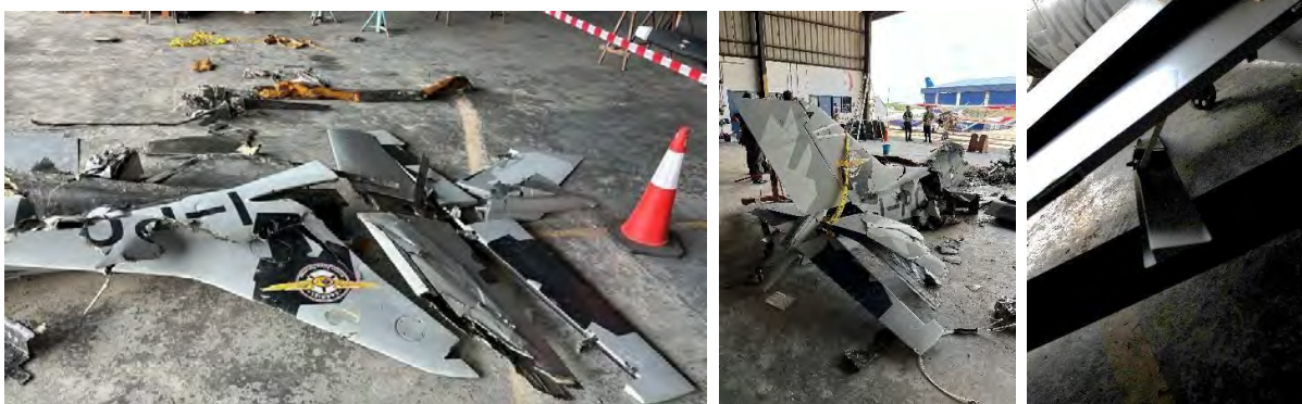
Figure 19. Tail Destroyed (Left), Tail Reconstructed (Middle), Trim Tab (Right)
