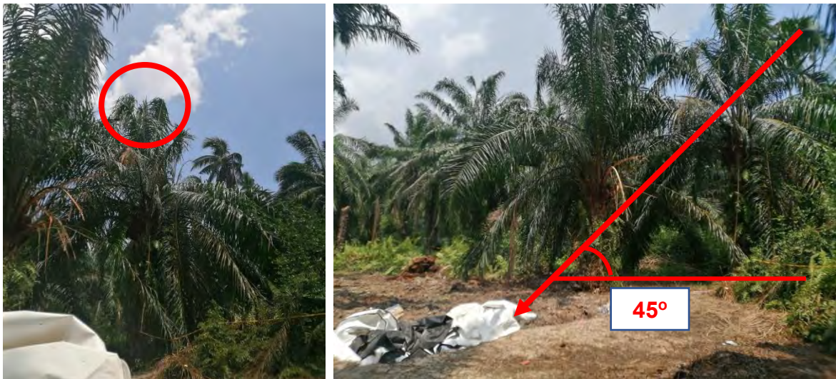
Figure 21. Broken Palm Branches (Left) and Aircraft Downwards Trajectory (Right)
