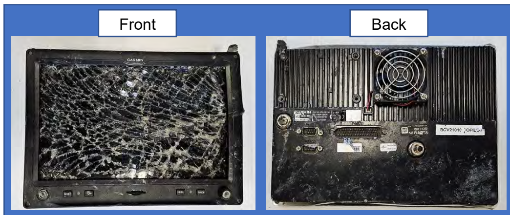
Figure 16. Damaged Garmin G3X GDU 460
