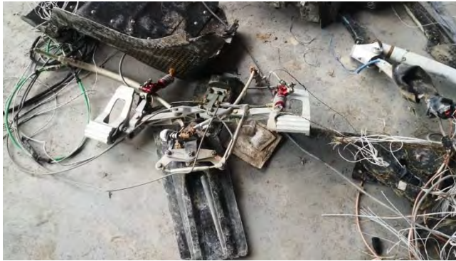
Figure 26. Rear Seat Rudder Pedal Relatively Intact
