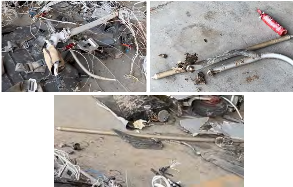
Figure 20. Longitudinal Control: Control Column (Top Left), First Connecting Rod (Top Right), Last Connecting Rod (Bottom)
