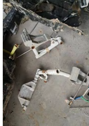
Figure 27. Pilot's Rudder Pedal Broken into Two Pieces
