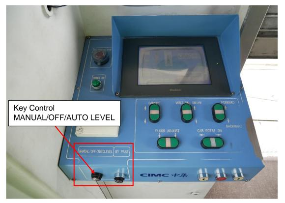
Figure 25: MANUAL / OFF / AUTO LEVEL Key Switch
