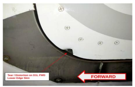
Figure 3: Damage forward passenger door lower edge skin.
