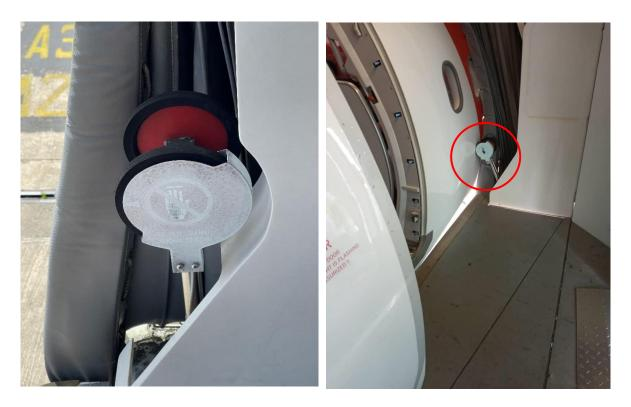
Figure 26: Auto Leveller retracted (Left) and extended to aircraft fuselage (Right) position
