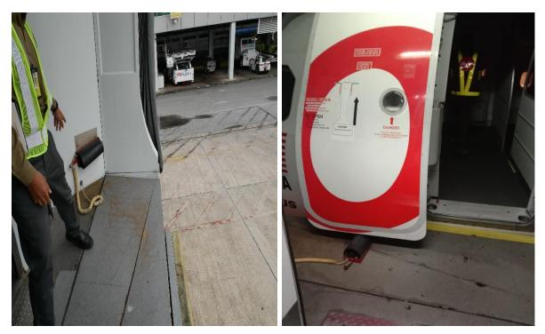
Figure 29: Safety shoe at stowed position (Left) and safety shoe placed below aircraft open door
