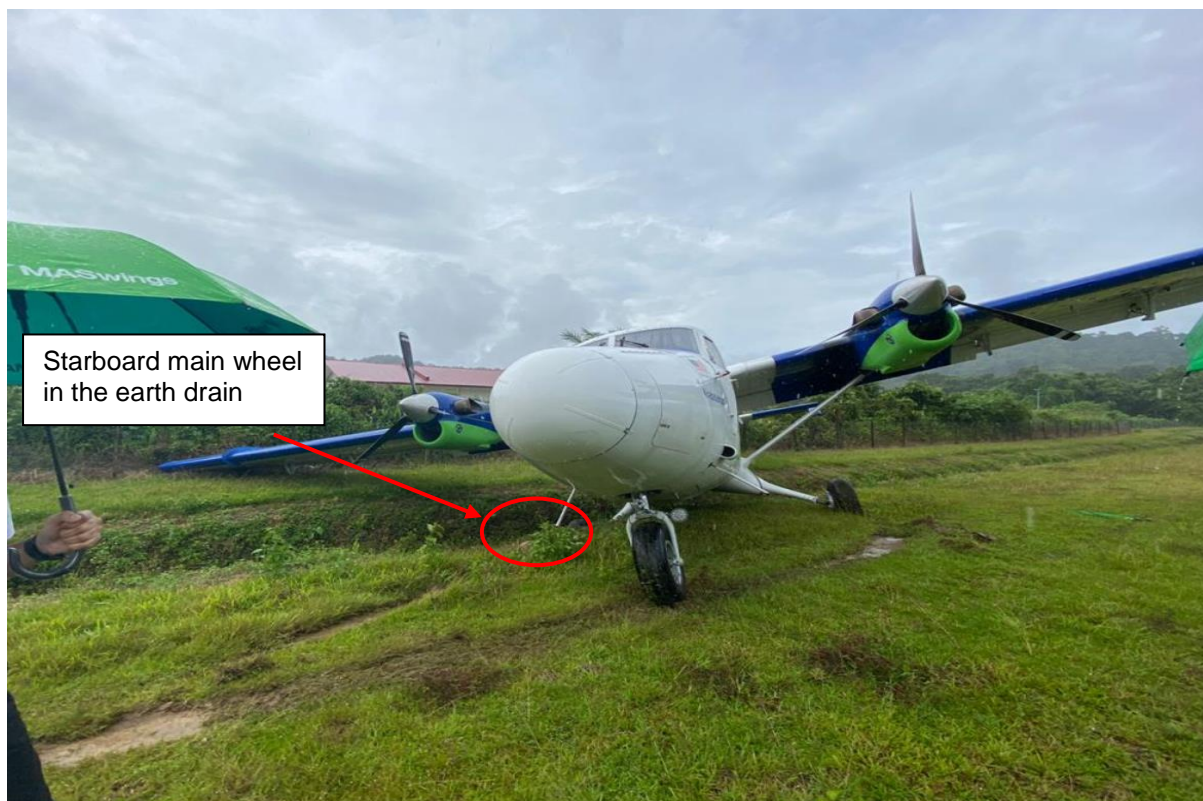
Figure 25: Aircraft final stop position after the starboard main wheel landed in the earth drain beside the runway.
