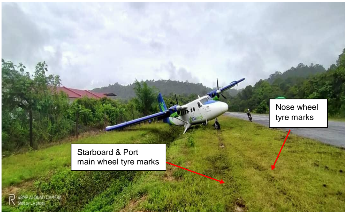
Figure 24: Aircraft continue with its forward momentum sliding sideways on the wet and soft ground to its final stop position facing close to the reciprocal heading of the landing direction.
