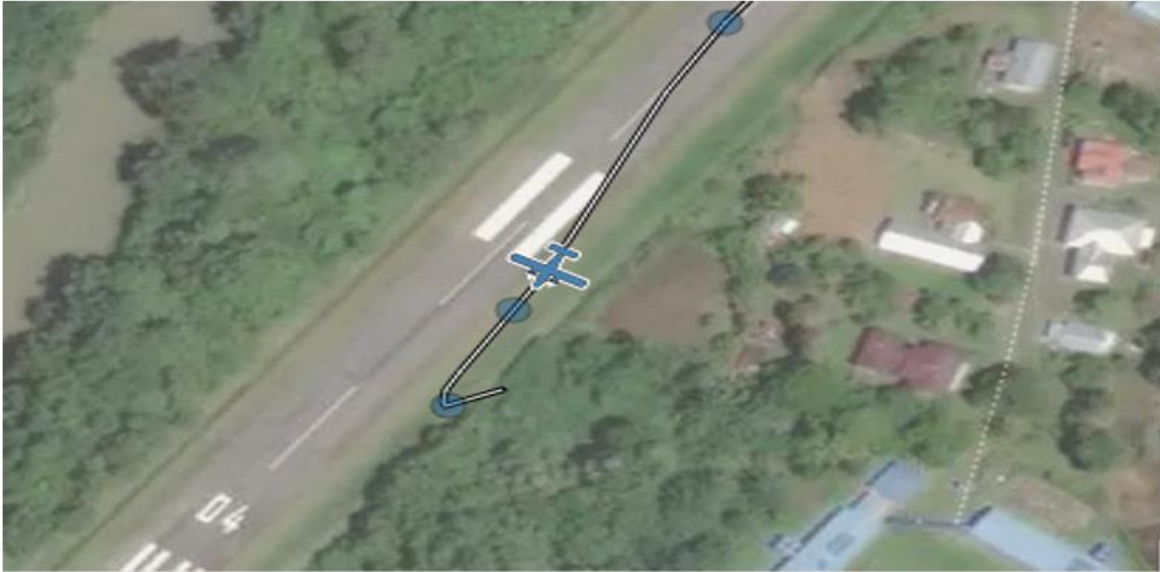
Figure 10: QAR data final approach to aircraft complete stop – aircraft veered left after touch down
