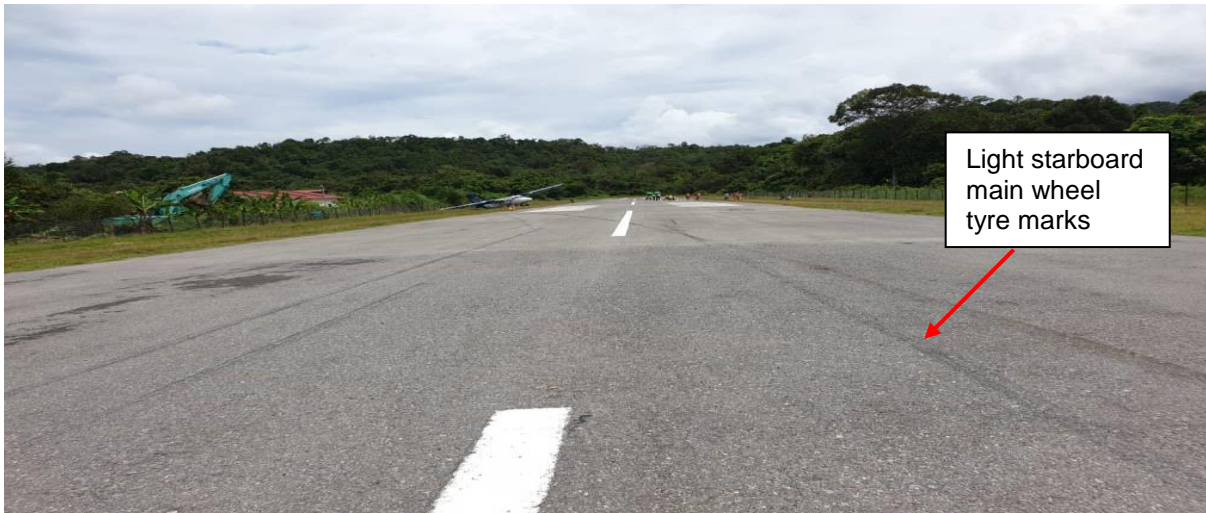
Figure 20: Aircraft landed on centreline and rolling straight after landing before starting to veered left. Pilot applied right rudder and right braking to counter left veering as seen in the initial light starboard main wheel tyre marks. No visible tyre marks for nose and port main wheel during initial veering.
