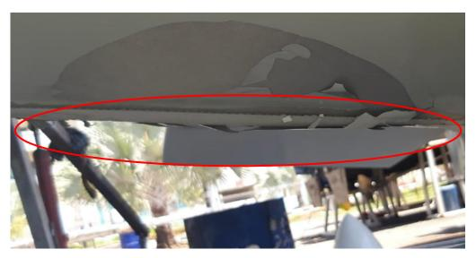
Figure 56: Bulged surface underside of lower right wing most probably caused by water impact at speed when right wing dropped into water creating a dragging force and veering the aircraft to the right
