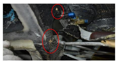
Figure 62: Patched repaired cracks at passenger seat frame still intact after accident (reverse side)
