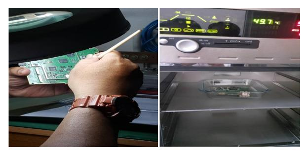
Figure 60: Cleaning and drying process of the GPS PCB at the laboratory
