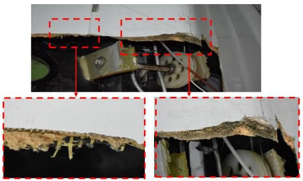
Figure 40: Fractured surface of the hull shows the impact was in the shear and tension mode
