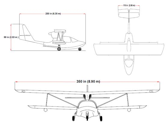
Figure 15: Three View of Aircraft
