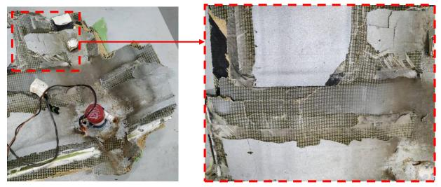
Figure 39: Delaminated & peeled off inner layer of the left hull
