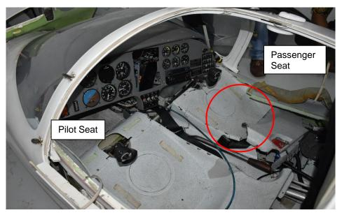
Figure 51: Pilot seat still intact while passenger seat broke and collapsed downward due to broken right hull during impact
