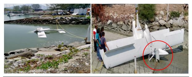
Figure 8: Aircraft wreckage was towed upside-down from the crash site to the marina ramp by a boat. Figure 9: Significant damage to the cockpit and nose section when the aircraft wreckage was lifted and lowered to the upright position by a crane.
