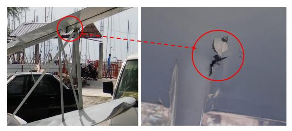
Figure 55: Torn skin underside of the upper right wing aileron fairing most probably caused by an object impact when right wing dropped and impacted the water
