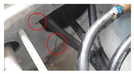
Figure 61: Cracks at passenger seat frame before accident
