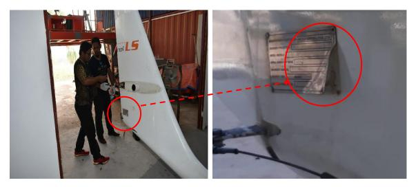
Figure 54: Aircraft registration metal plate on the right tail fuselage section dislodged most probably caused by either boat towing or crank lifting process during salvage operations
