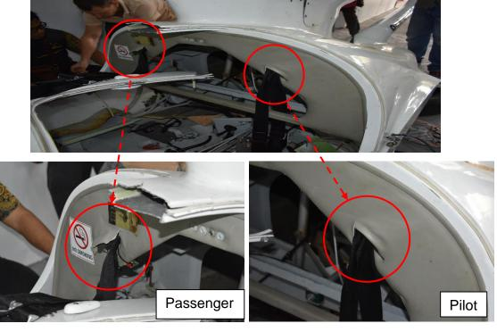
Figure 49: Passenger seat belt harness<br/>frame crack due to rapid deceleration G<br/>forces during impactFigure 50: Pilot seat belt harness frame<br/>in good condition
