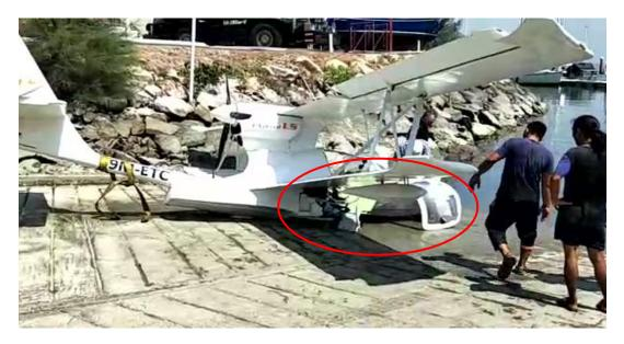
Figure 10: Aircraft wreckage in upright position with fuselage broken into two pieces. Cockpit area and nose section heavily damage during lowering process by the crane onto the ramp.
