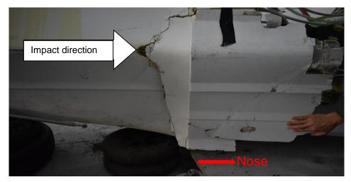
Figure 41: Impact mark on the centre bottom aft hull
