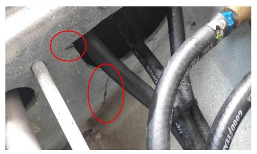
Figure 21: Crack under passenger seat frame.
