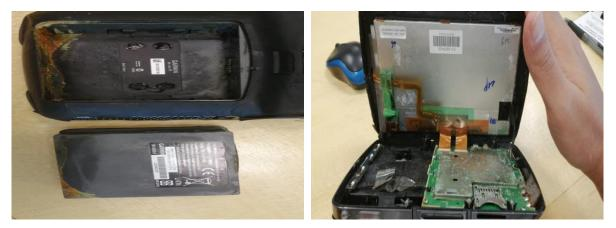
Figure 59: Condition of the GPS after recovery from the wreckage
