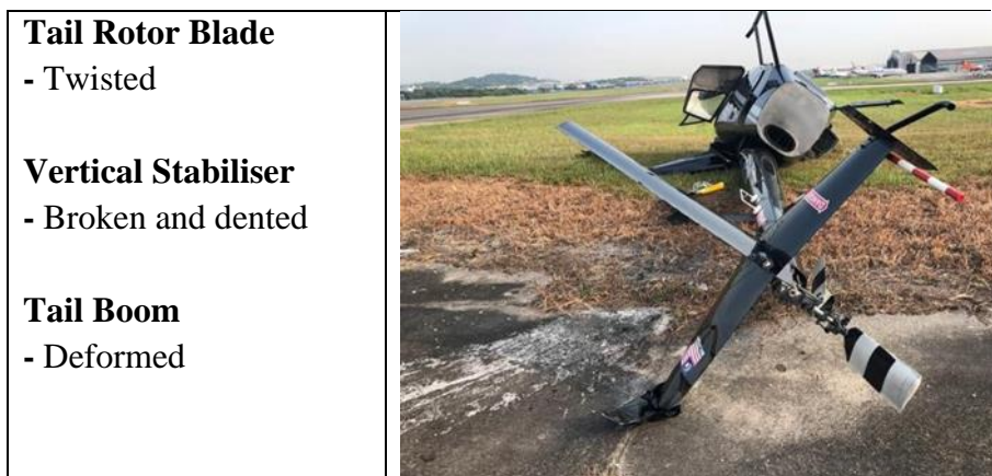
Figure 7: Tail rotor blade, vertical stabiliser and tail boom
