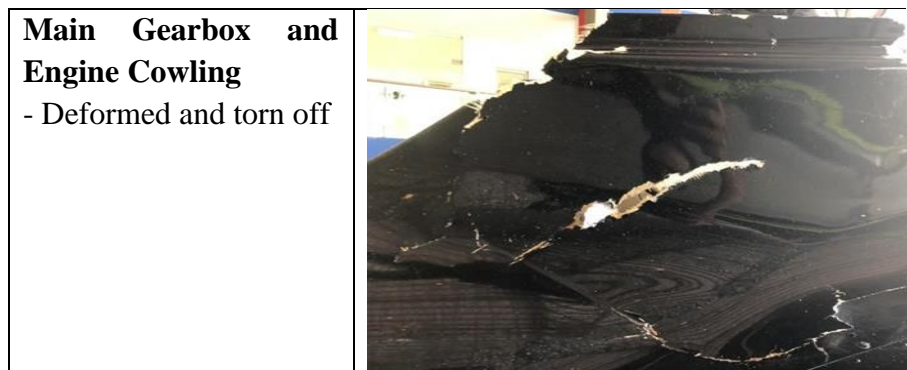
Figure 10: Main gearbox and engine cowling
