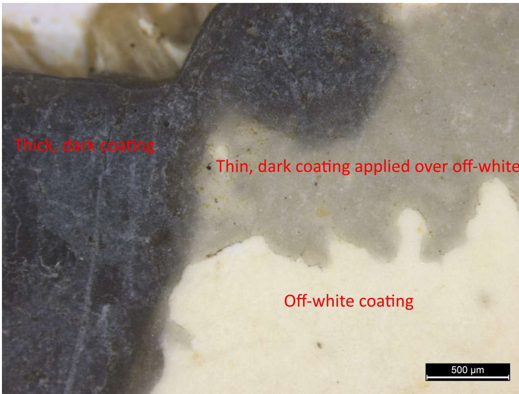
Figure 4: Close-up of applied coatings
