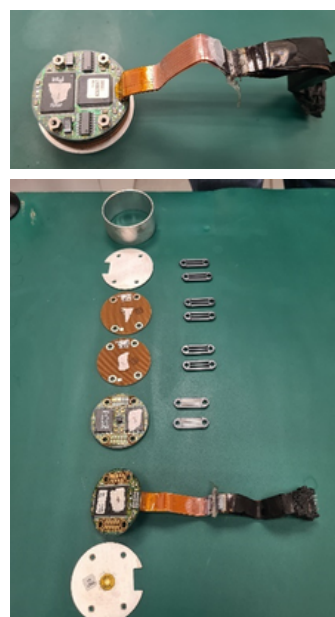
Top: Memory puck with its base cover removed, showing the memory PCB. This puck was in good condition. Only the ribbon cable exhibited thermal damage from exposure to the post-crash fire.
