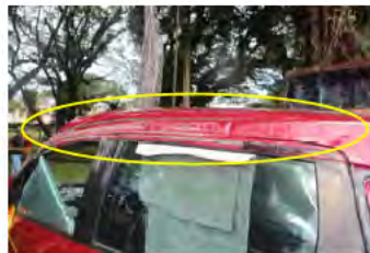
Multiple direction scratches on both nearside and offside upper structure of the Alza, along with a collapsed front roof and deformation of A-pillar, strongly indicate the multiple rollovers occurred.
