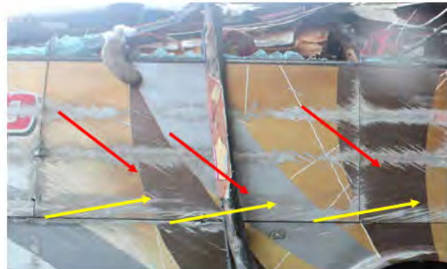
Dual direction scratch marks – ▪ sliding motion forward ▪ Directional change – rotation anticlockwise due to pulling effect by penetrated railings
