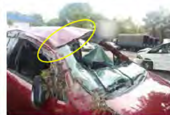
Multiple direction scratches on both nearside and offside upper structure of the Alza, along with a collapsed front roof and deformation of A-pillar, strongly indicate the multiple rollovers occurred.
