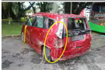
The nearside rear structural deformation was caused by the contact with the embankment before the Alza came to a complete stop.
