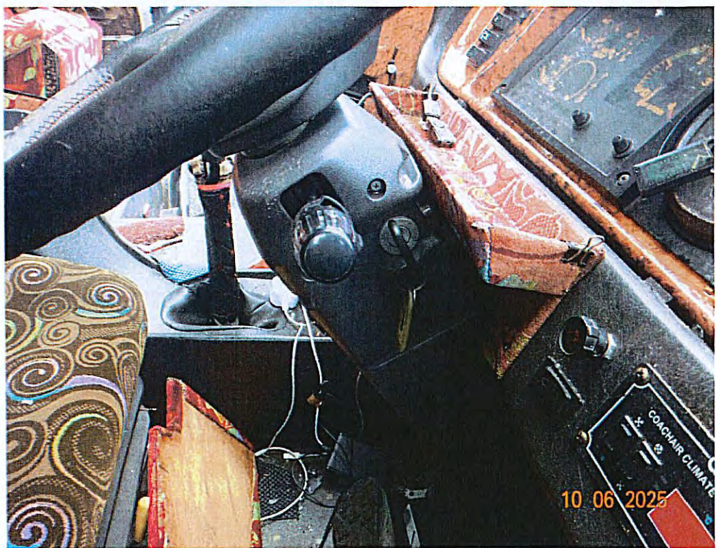
SISTEM STEERING: STEERING COLUMNS SHAFT
