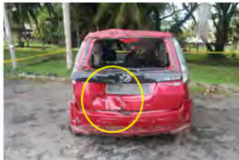
The rear-end structural deformation was caused by the impact force by the Bus.
