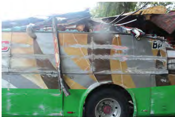
3 glaring scratch marks – due to support frame underneath body as the Bus skidded and rotated
