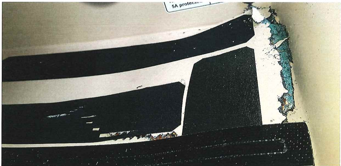
Picture 3 show the extensive damage of the crack, view inside of the cabin on the Pilot side (Left-hand seat).
