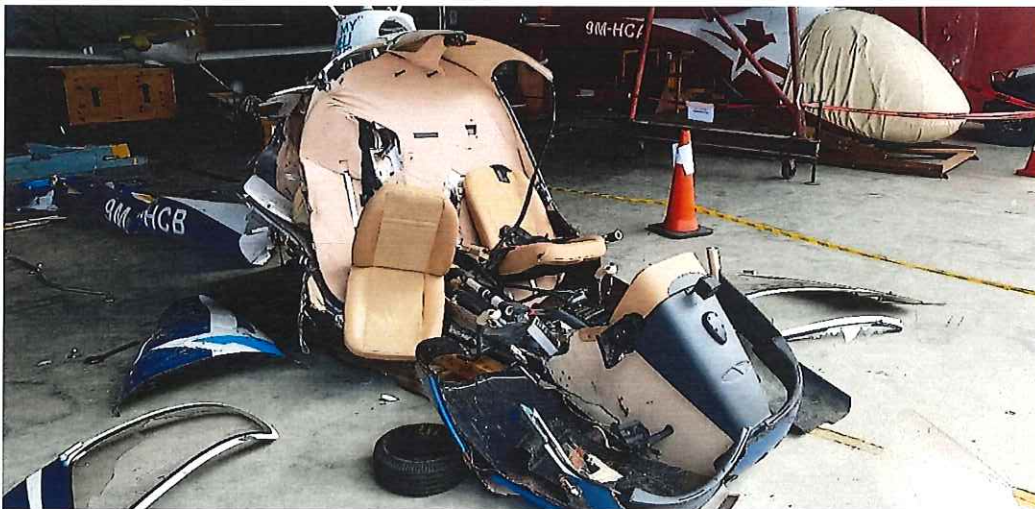
Picture 1 shows the extensive damage of the front section of the fuselage. The windscreen and the doors of the aircraft were found detach at the crash site.
