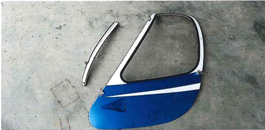
Picture 12 shows the left-hand side door with the left-hand side of the front member of the forward fuselage. These parts were found detached from the aircraft and were recovered at the crash site.
