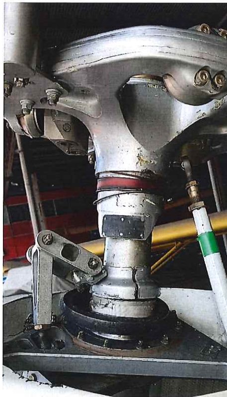
Picture 31 shows the extensive damage to the main rotor head. Shown in this picture the upper scissors fittings rivets are sheared off from the rotor head. Can be seen also the droop stop ring were detached from the main rotor head. All of the pitch links and main rotor blades were removed for ease of transportation from the crash site.
