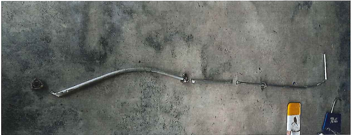
Picture 24 shows the broken pieces of the tail rotor driveshaft. Most of the driveshaft found evidence of torsional and shear damage. Can be seen also in this picture the hanger bearing that is detached from the aft engine firewall and were recovered at the crash site.
