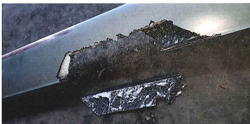
Picture 37 shows the broken portion of the trailing edge of the green main rotor blade.
