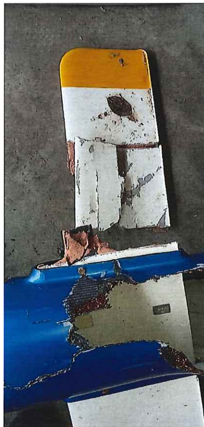
Picture 19 shows the broken horizontal stabilizer view from above.
