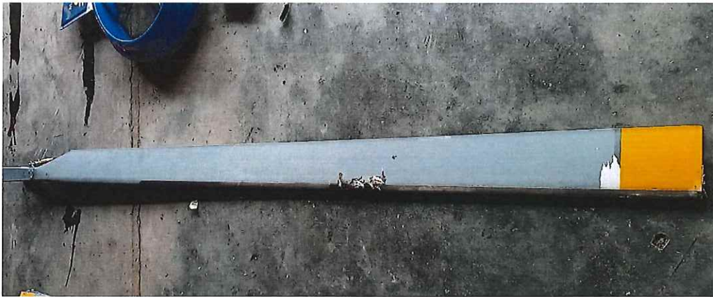
Picture 32 shows the yellow main rotor blade of the aircraft. The blade suffered substantial damage to the leading edge of the blade and delamination. The lead-lag damper was found detached from its body.
