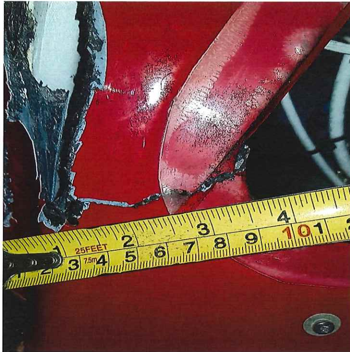
Picture 8 shows crack on the fuselage adjacent to the punctured area. Measurement of the crack is roughly 3.5 inches. View is taken from the left-side of the fuselage. (Near to left engine cowl door latch).
