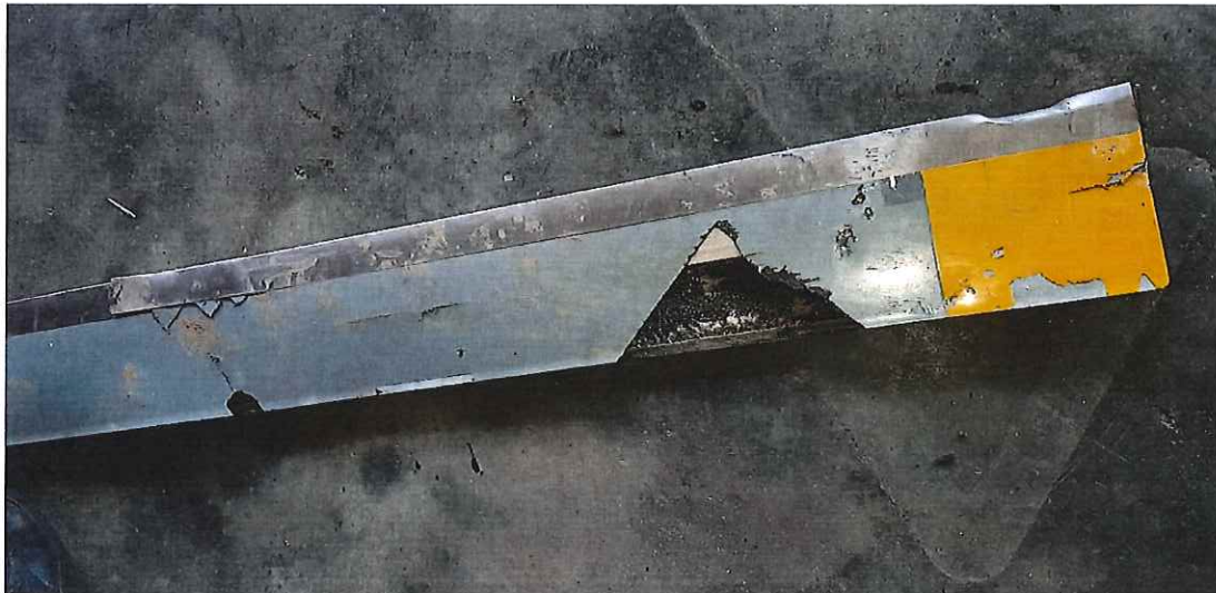
Picture 41 shows the damaged tip of the red main rotor blade. Can be seen in this picture also missing portion on the trailing edge of the blade.
