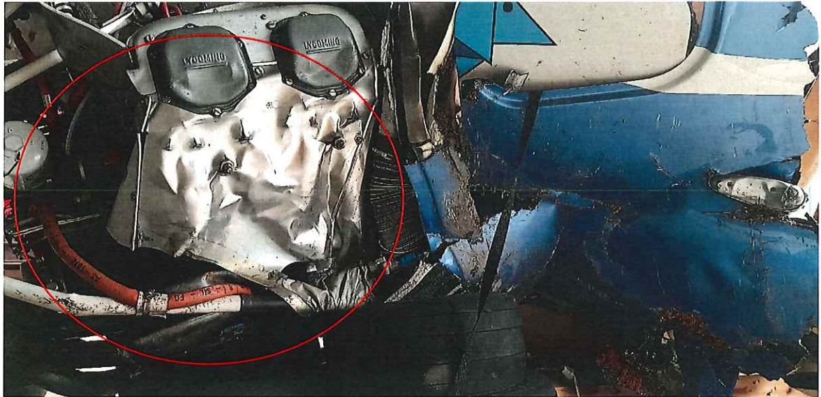
Picture 8 shows the right-hand side of the engine. Shown in the circle in this picture are the damaged lower engine baffled and the bent left-hand engine truss.
