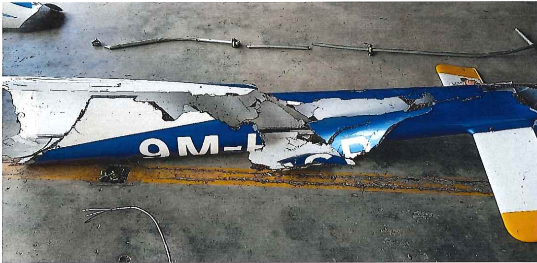
Picture 18 shows the left-hand side of the tail boom. Can be seen in this picture most of the tail boom are broken to several pieces.
