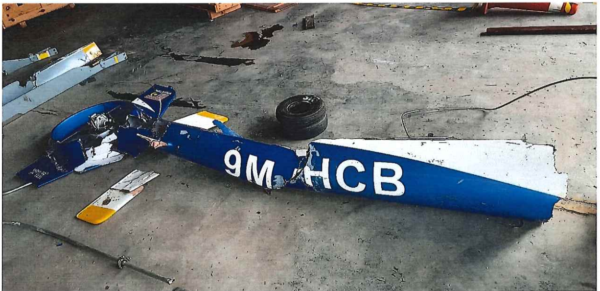
Picture 17 shows another angle of the broken tail section. Can be seen in this picture the broken right-hand side of the horizontal stabilizer.
