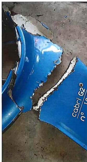
Picture 21 shows the broken lower fin of the tail section of the aircraft.
