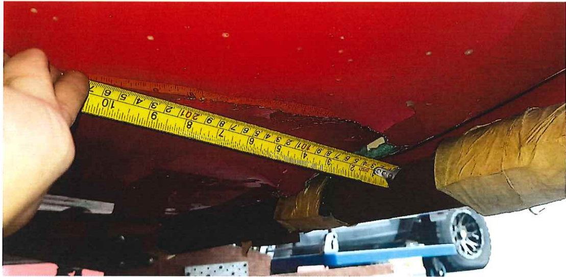
Picture 2 shows the measurement of the crack along the fuselage is at 8.7 inches.
