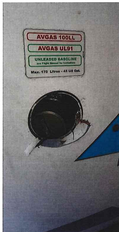
Picture 11 shows the left side of the aircraft where the fuel bladder is position. Can be seen the fuel cap is still attached to the fuel bladder and has move inwards into the fuselage. The fuel bladder is still intact, and no leak was found.
