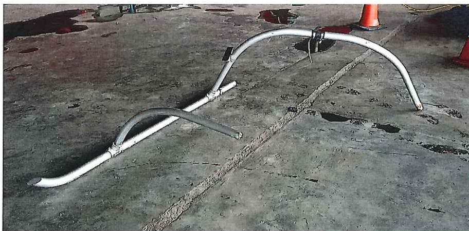
Picture 11 shows the condition of the aircraft skid after the incident (the left-hand skid missing)
