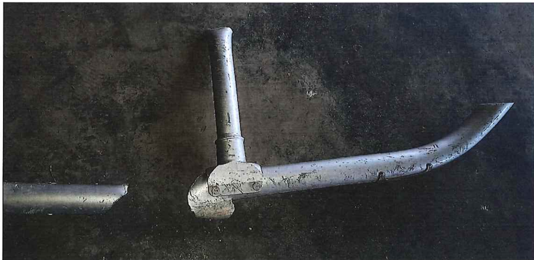
Picture 27 shows the broken piece of the right-hand skid assembly.
