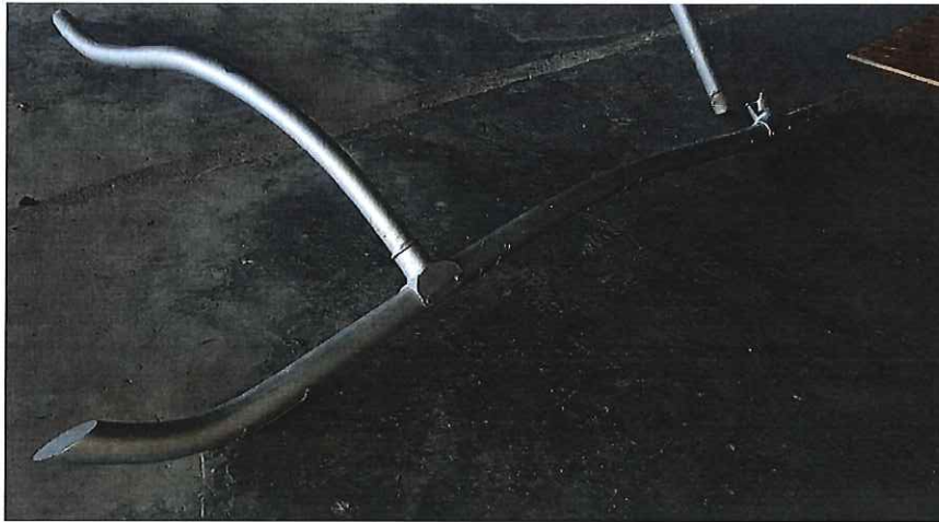
Picture 30 shows the left-hand skid of the landing gear assembly. Shown in the picture the landing gear is bent and the rear bow is detached from the attachment to the skid.
