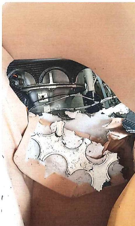
Picture 7 shows the broken wall section of luggage compartment. Can be seen in this picture the main gear box of the aircraft.
