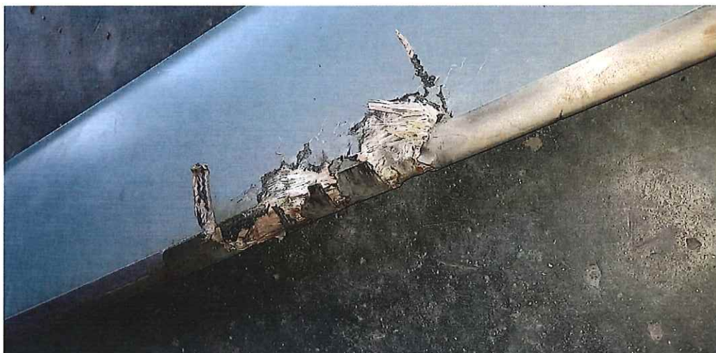
Picture 35 shows the damage portion of the leading edge of the yellow main rotor blade.
