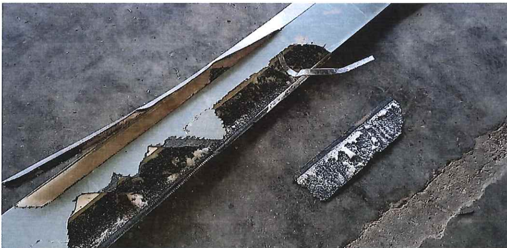
Picture 40 shows the damaged leading and trailing edge of the red main rotor blade.
