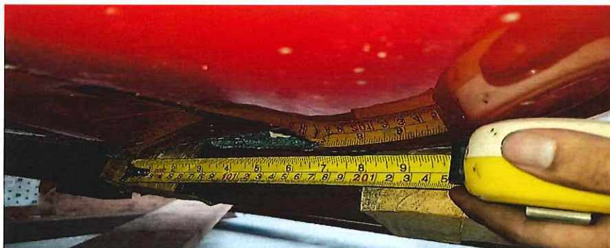
Picture 1 shows the crack on the Right-hand side of lower fuselage looking from aft of the aircraft. Measurement of the crack spanwise is at 7 inches.
