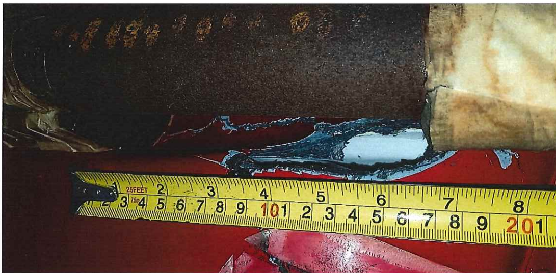
Picture 7 shows the aft left-hand lower fuselage punctured found during inspection. The hole is measured roughly at 4 inches spanwise. Length including the crack spanwise is roughly at 8 inches.
