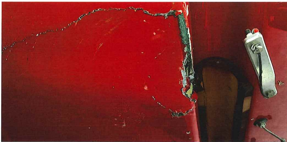
Picture 5 shows the damage on the lower fuselage structure (top view). The bent ATC transponder antenna could be seen on the lower left side of the picture.
