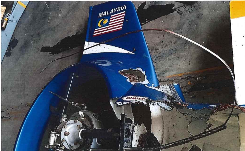
Picture 25 shows the damaged tail rotor cable. Half portion of the cable are found still attached to the fuselage of the aircraft. Can be seen also in this picture the damaged fin of the aircraft.
