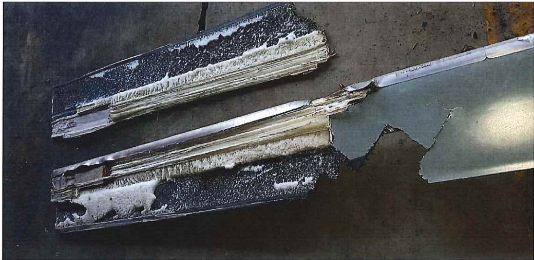
Picture 38 shows the broken piece of the upper section of the green main rotor blade. Some portion of the trailing edge also can be seen missing from the blade.
