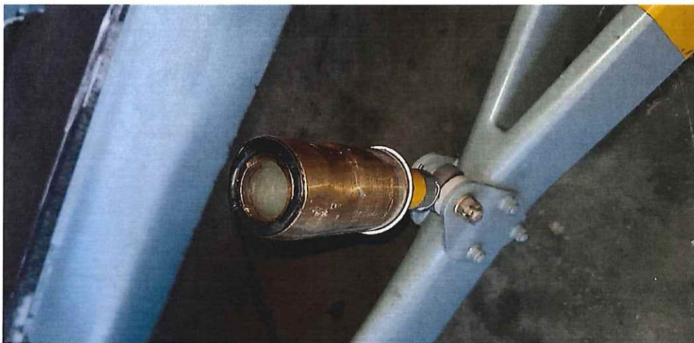
Picture 33 shows the half portion of the yellow lead-lag damper that is found detached from the body.
