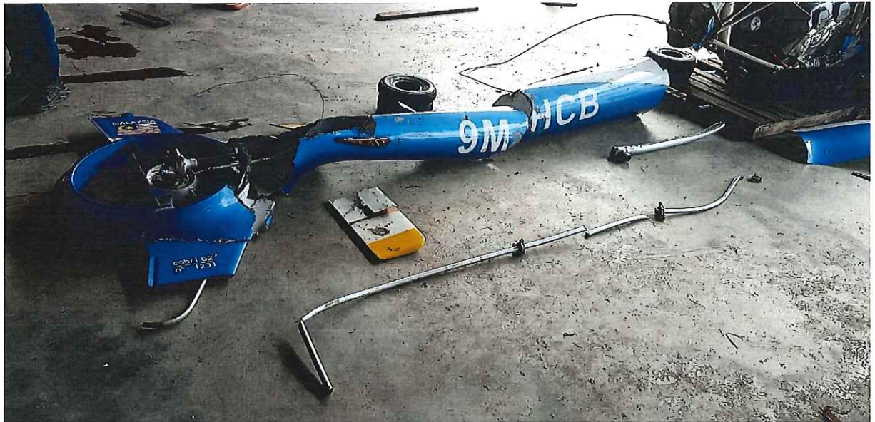
Picture 16 shows the tail section and the tail driveshaft of the aircraft. Most of the tail section are broken and were recovered at the crash site.
