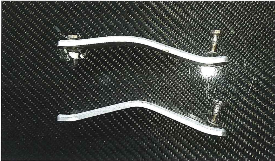
Picture 6 shows the two-damaged front cross tube attachment bars of the aircraft.
