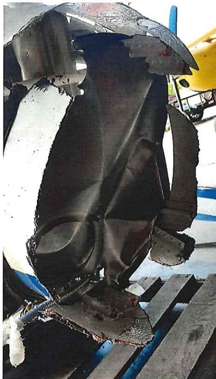
Picture 15 shows the aft engine firewall of the aircraft. Can be seen in this picture the tail attachments of the aircraft still attached to the truss structure.
