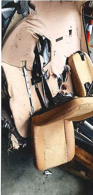
Picture 4 shows the pilot seat are mostly detach from the rails on the wall of the cabin. Can be seen in the picture also most of the right-hand side of the lower fuselage are destroyed due to the crash.
