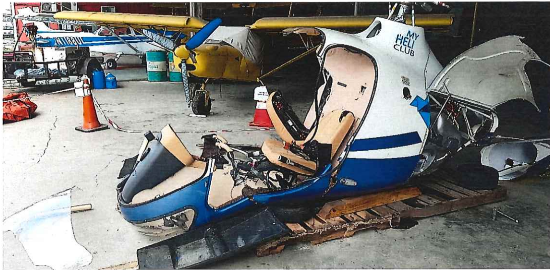
Picture 10 shows the left-hand side of the aircraft fuselage. In comparison to the left side, most of the structural parts of the aircraft are still attached. Can be seen in this picture, the co-pilot seat is still attached to wall of the cabin.
