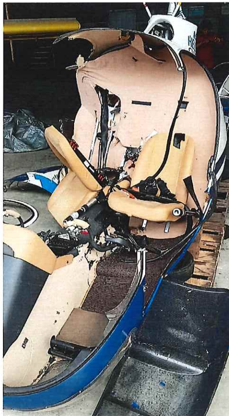
Picture 13 shows the front portion of the left-hand side of the aircraft. Can be seen in this picture the damaged center pedestal and detached pilot seat.
