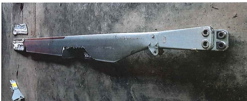
Picture 36 shows the green main rotor blade of the aircraft. Substantial damage on the blade could be seen in this picture
