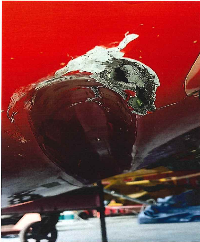
Picture 10 shows the hole from the left-hand side of the fuselage body adjacent to the skid attachment.
