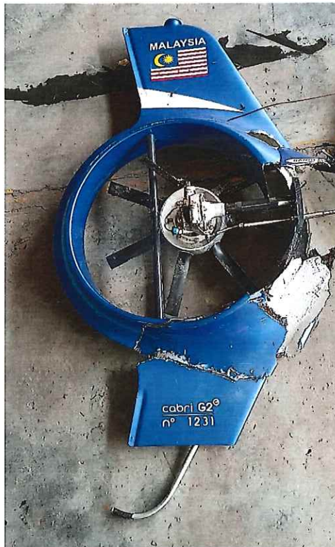
Picture 20 shows the fenestron of the aircraft. Can be seen in this picture most of the fin structure was broken and were recovered at the crash site.
