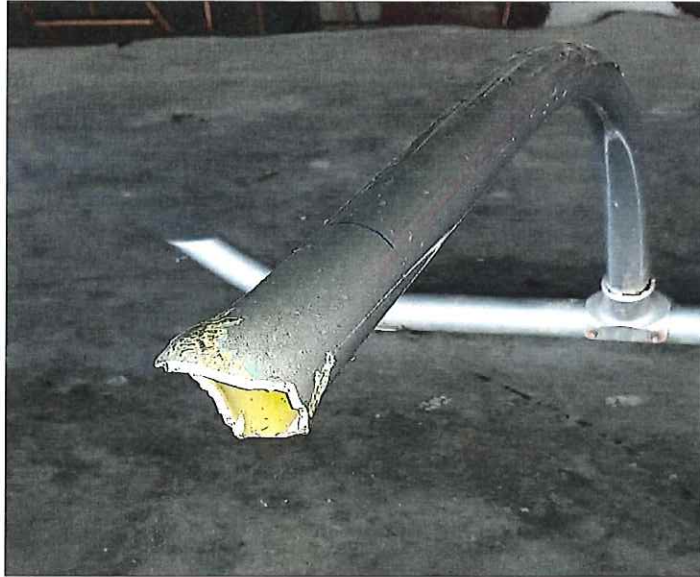
Picture 12 shows the damage on the Left-hand side forward cross tube on the landing gear.
