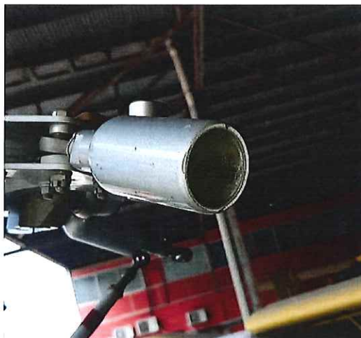
Picture 34 shows the body of the yellow lead-lag damper still attached to the main rotor head.
