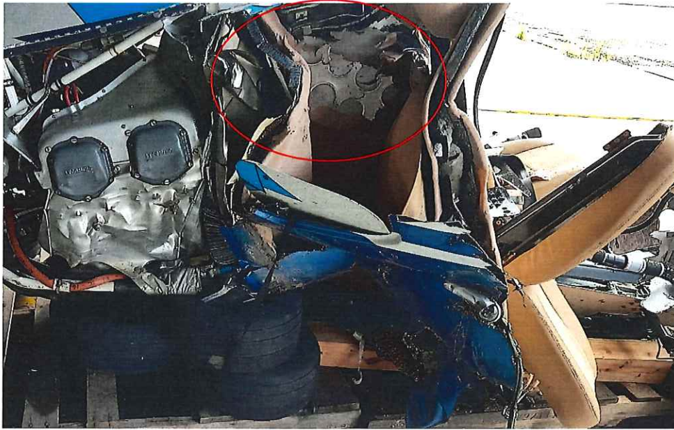
Picture 6 shows the right-hand side of the aircraft fuselage. The circle shown in the picture shows the damage luggage compartment of the aircraft. Some portion of the main gearbox could be seen also in this picture.
