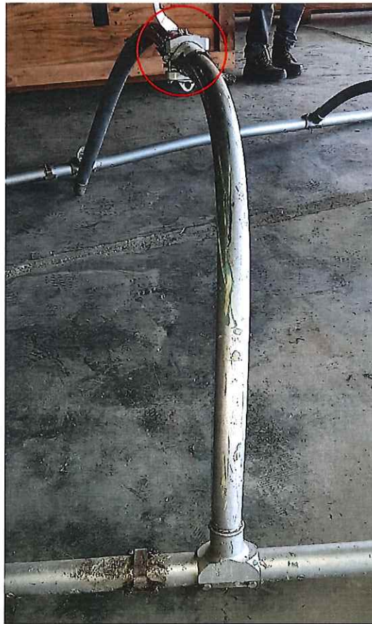
Picture 28 shows the aft bow of the landing gear assembly. Shown in the circle the rear bow attachment to the fuselage detached from the lower fuselage.
