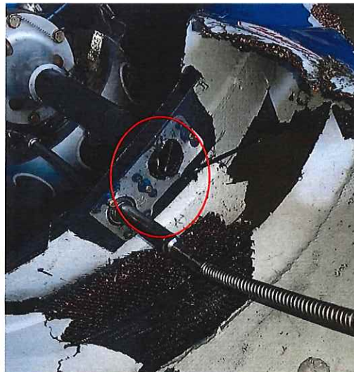
Picture 23 shows broken section of the entire fin. The circle shown in the picture shows the sheared portion of the tail rotor driveshaft.
