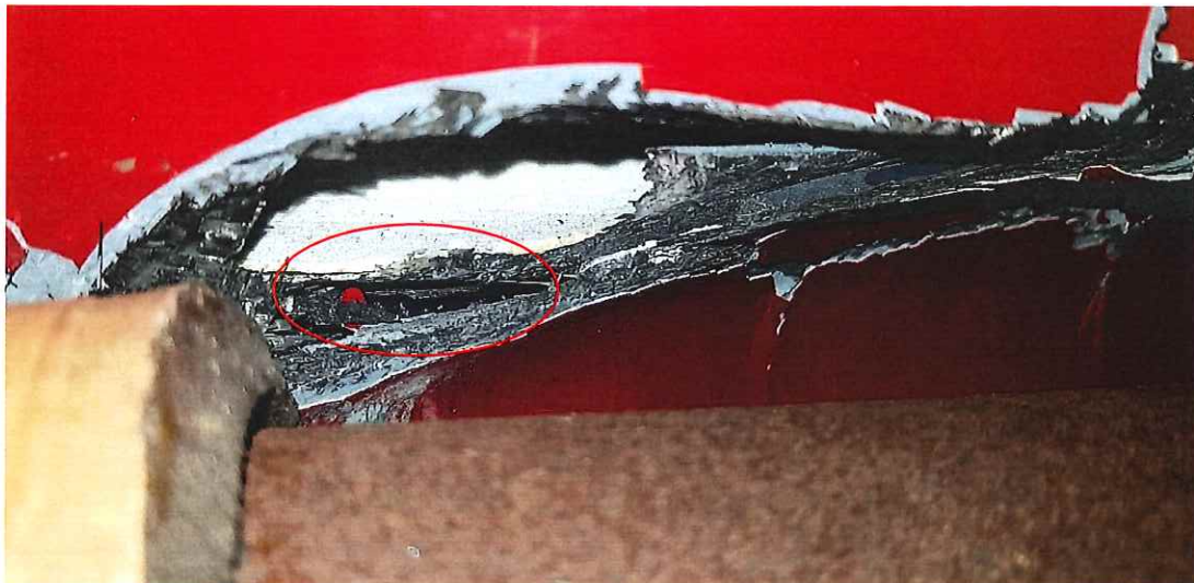
Picture 9 shows the view from aft to forward of the aircraft. The circle shown the area where the fuel bladder cell is slightly visible from the outside.
