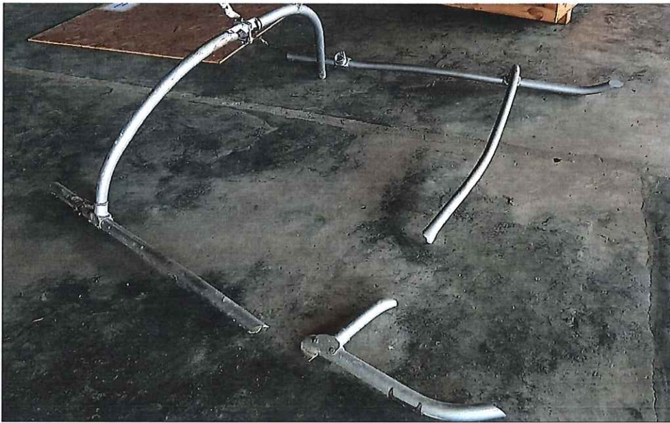
Picture 26 show the broken landing gear of the aircraft. Can be seen in this picture the landing gear are broken to 3 pieces. All the broken pieces were recovered from the crash site.
