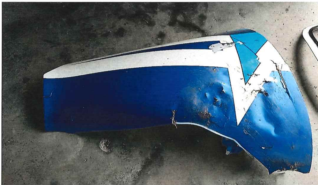
Picture 9 shows damaged right-hand side of the engine cowling.
