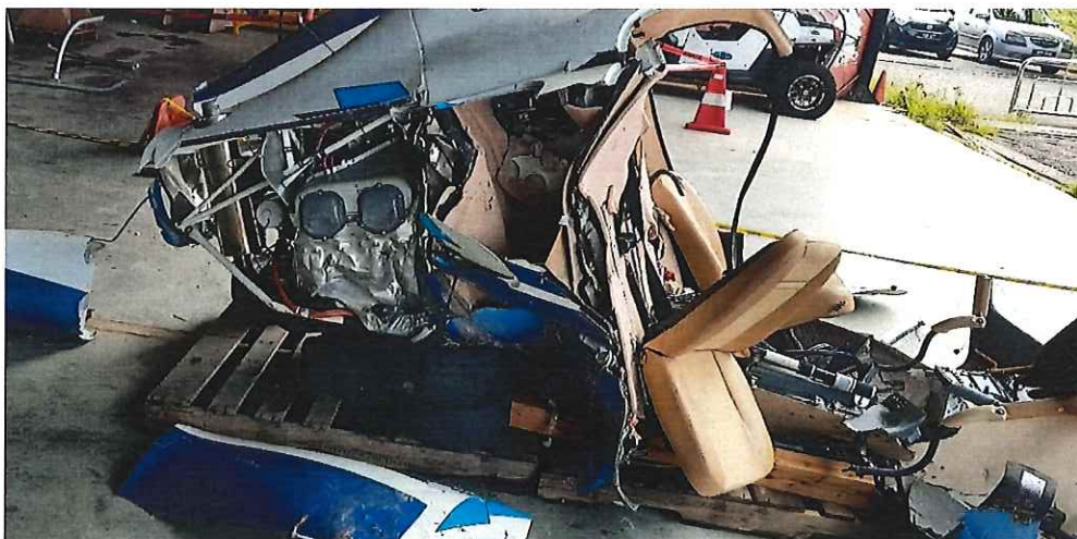
Picture 5 shows the right-hand side of the of aircraft fuselage. Most of the sections were destroyed due to the crash. Shown in the picture the right-hand engine cowling.
