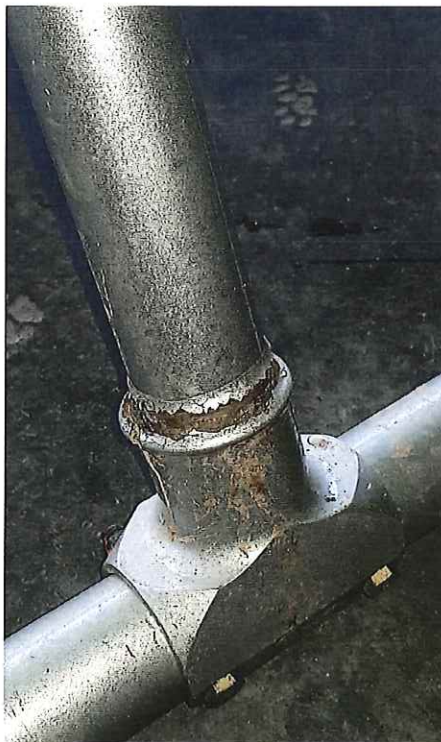
Picture 13 shows the damage on the right-hand side of the forward cross tube attachment to the right-hand skid.
