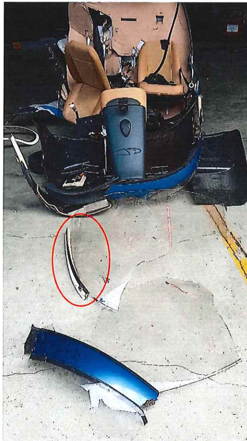
Picture 2 shows the portions of the windscreen and the forward left-hand side of the fuselage. Shown in the circle are the forward right-hand member of the front portion of the fuselage.
