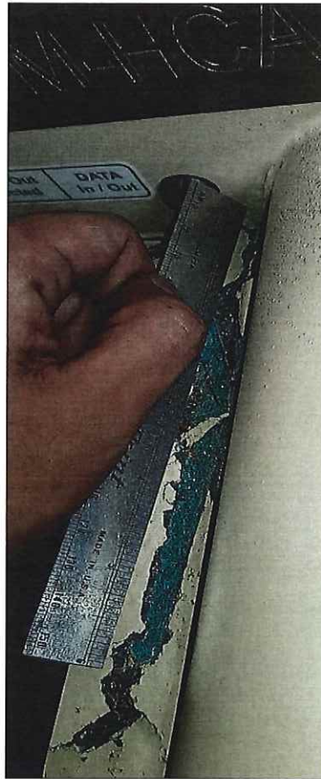
Picture 4 shows the measurement of the crack view from inside of the cabin is measured more than 6 inches. (Measurement taken show 7 inches).
