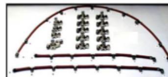
Flexible Manifold Conf. (Post-SB21705) - 43 detail parts
