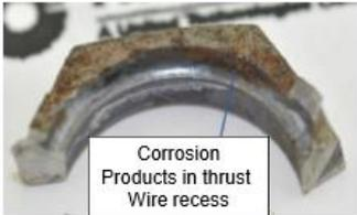
Corrosion Products in thrust Wire recess
