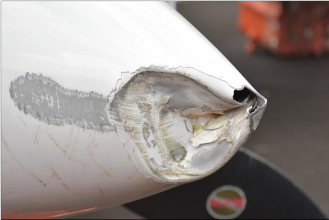
Picture 5 – Propeller spinner dented
