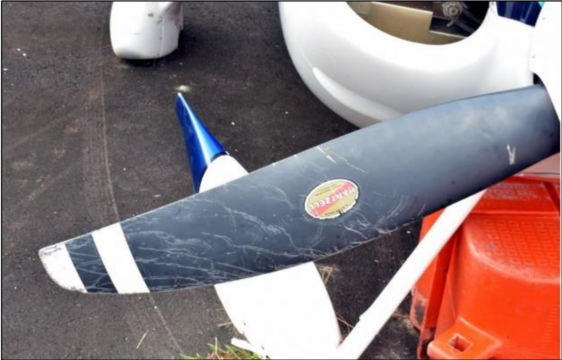
Picture 6 – Propeller Strike
