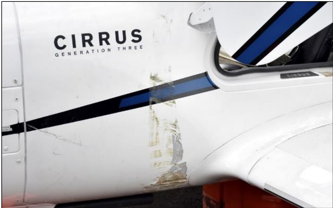
Picture 7 – Dented and minor scratches on the fuselage
