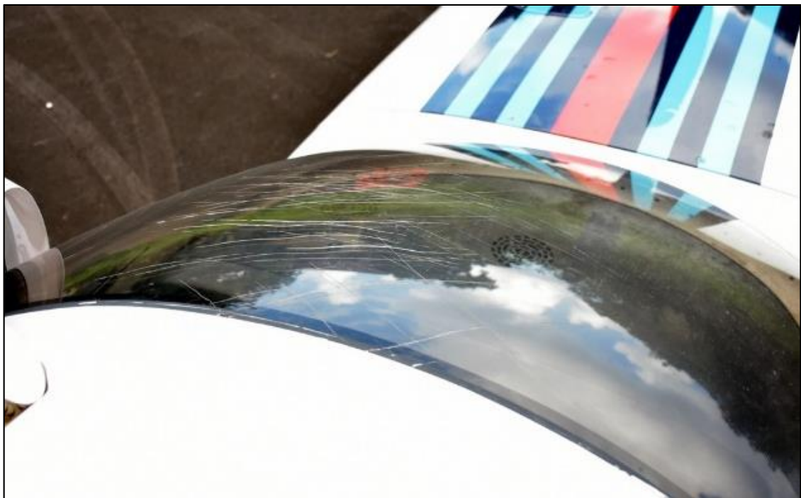
Picture 8 – Scratches on the windscreen
