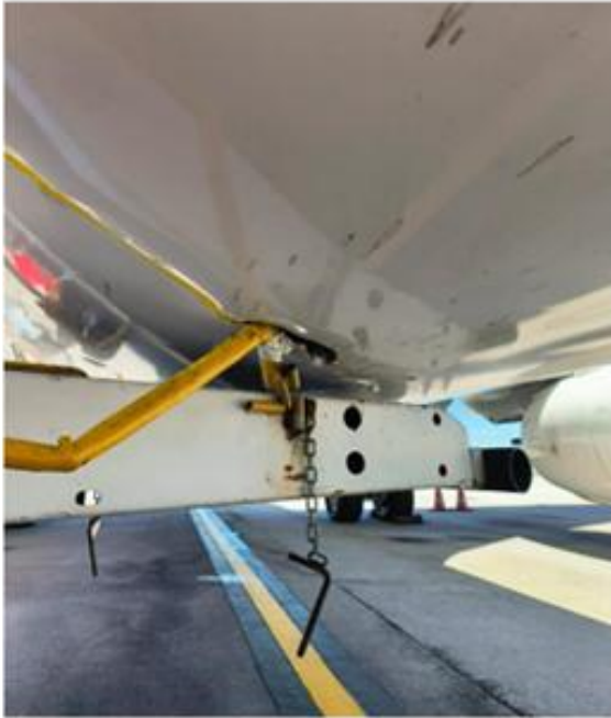
Belt loader conveyor handrail contacted A/C fuselage
