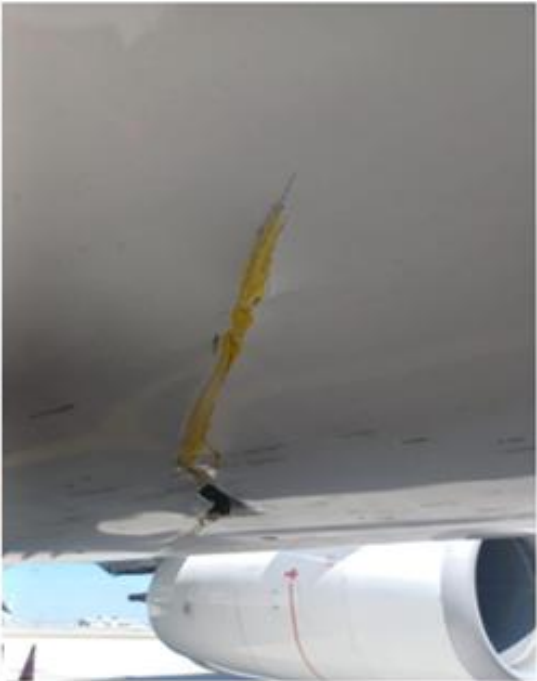
Damage on the lower sector of the a/c fuselage
