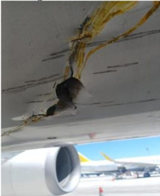
Damage on the lower sector of the a/c fuselage
