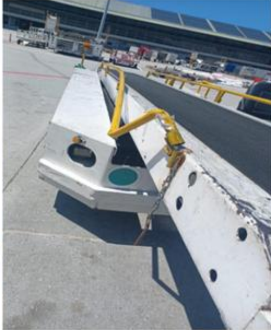
Damage on the Belt loader conveyor handrail
