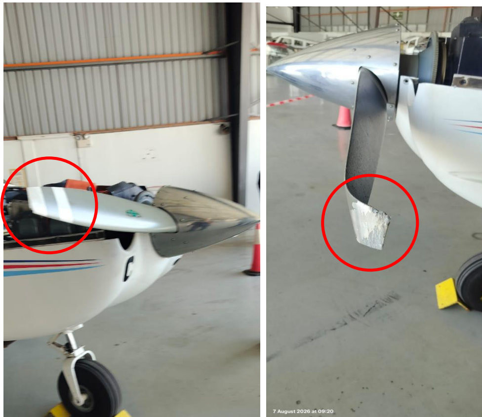
Figure 2: Condition of propeller blade tips.
