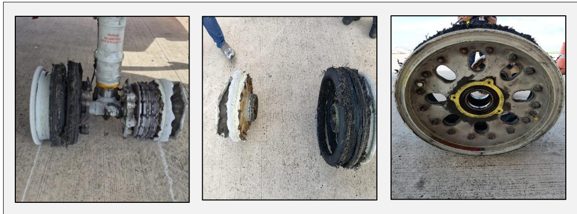
Figure 6: MWA No. 3 & No. 4 Damaged
