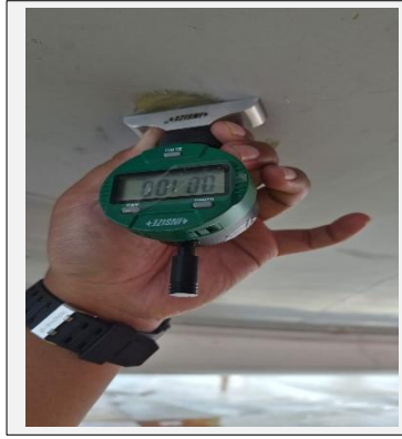
Figure 13: RH Inboard Lower Tank Dented
