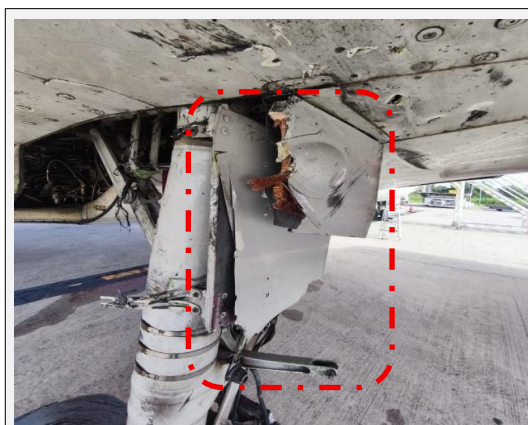
Figure 19: RH Outer, Centre and Inner Doors Main Landing Gear Broken and Fractured
