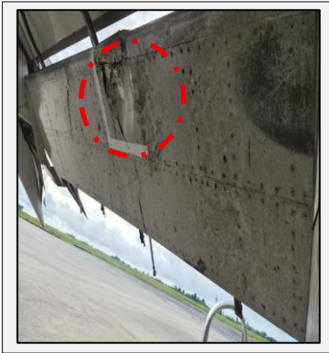
Figure 12: RH Inboard Trailing Edge Flap Dented
