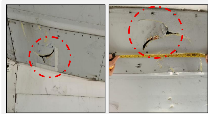
Figure 15: RH Aft Lower Wing Root Panel Ruptured
