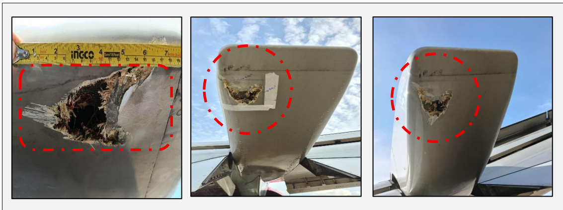
Figure 7: RH Canoe No 4 Ruptured
