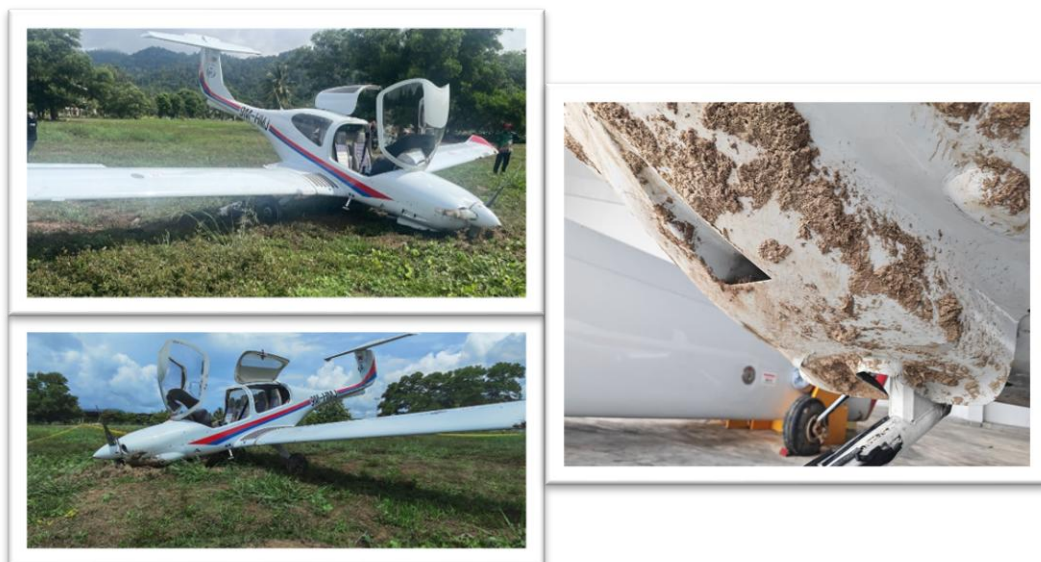
Figure 5 : Condition of Lower Fuselage (Nose Wheel Fuselage)
