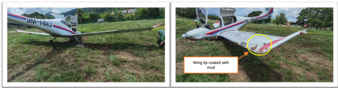
Figure 6 : Condition of Wings and Empennage
