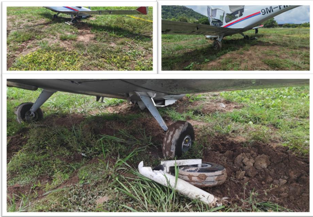
Figure 3 : Condition of Main Landing Gear
