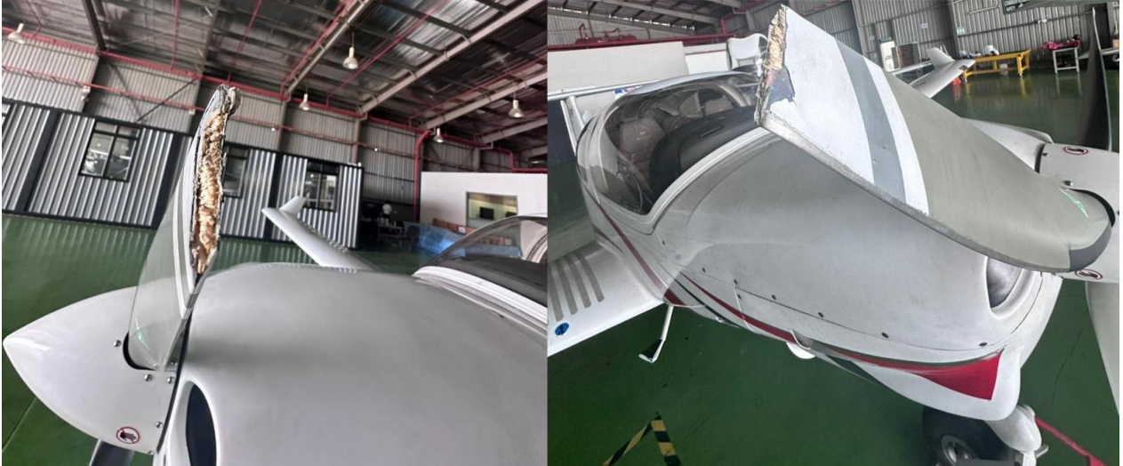
Figure 2: Condition of propeller blade tip.
