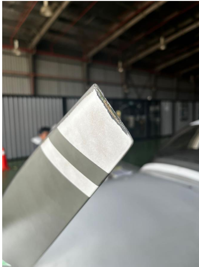
Figure 3: Condition of propeller blade tip.
