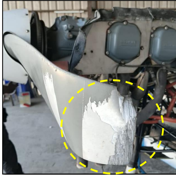
Figure 1: Condition of the aircraft propeller blades
