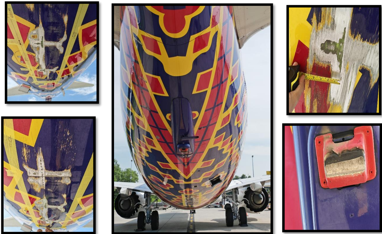
Figure 1: Tail Strike Damage to the Lower Aft Fuselage
