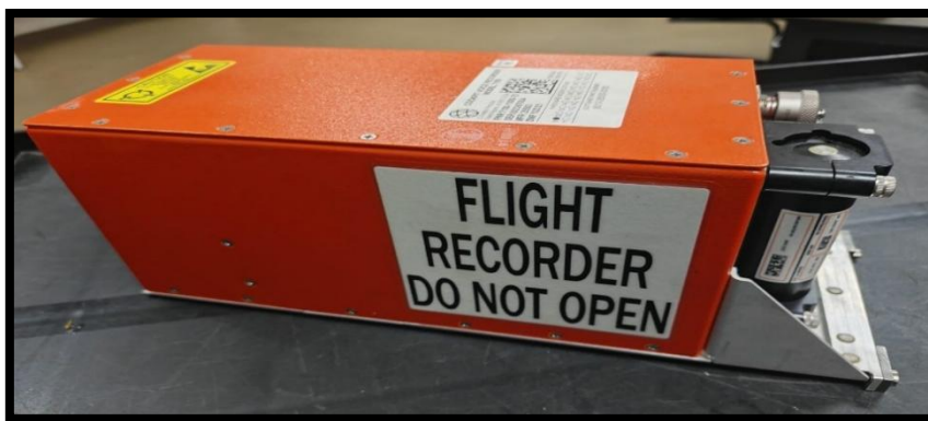
Figure 4: Cockpit Voice Recorder (CVR), Model 7100
