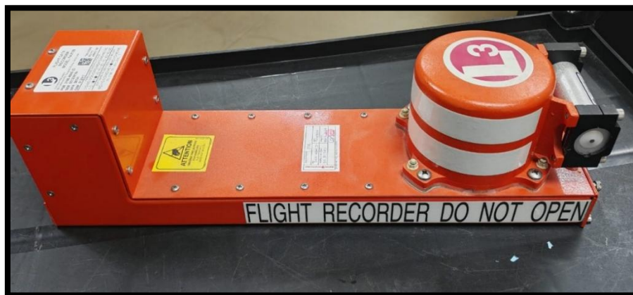
Figure 3: Flight Data Recorder (FDR), Model FA2100
