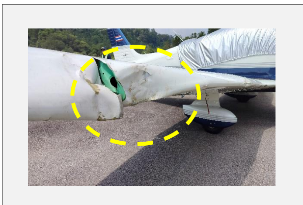
Figure 5: Side View – RH Wing Leading Edge damage area
