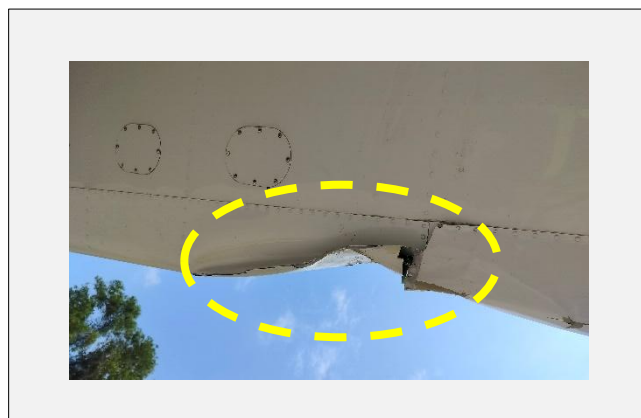
Figure 6: Bottom View – RH Wing Leading Edge damage area
