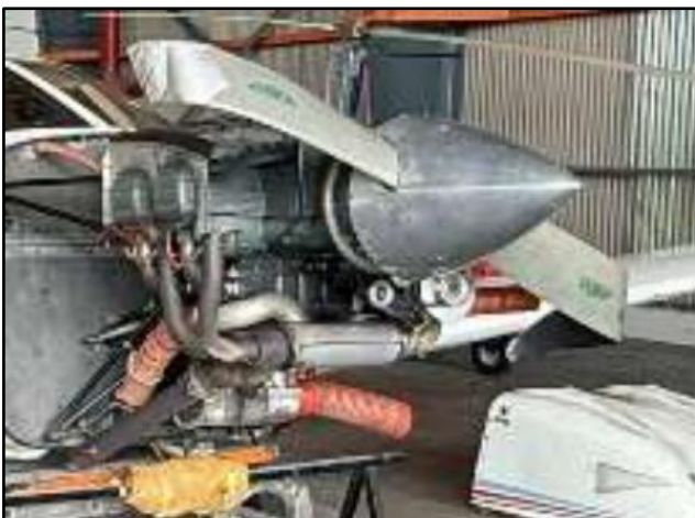
Figure 4: As specified in Lycoming's mandatory service bulletin SB533C, any sudden engine stoppage or propeller strike should be removed and engine shock load called for.
