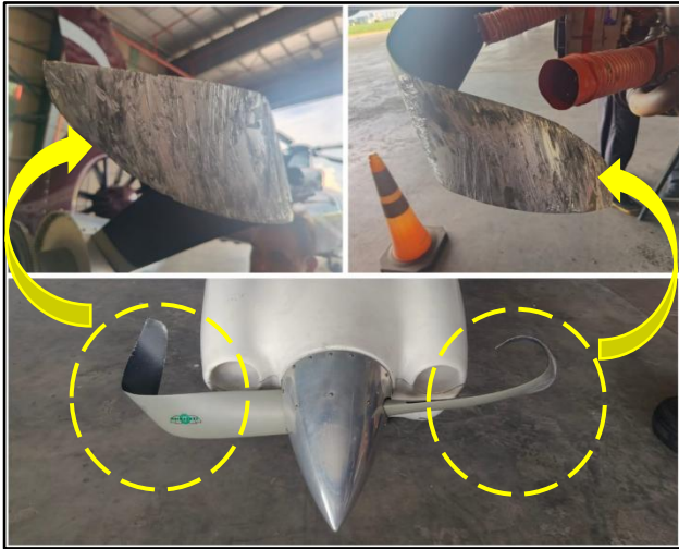
Figure 1: Condition of the aircraft propeller blades
