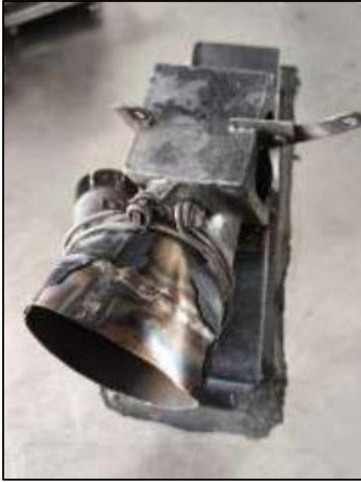
Figure 7: The box assembly was severely damaged, and a dent was observed
