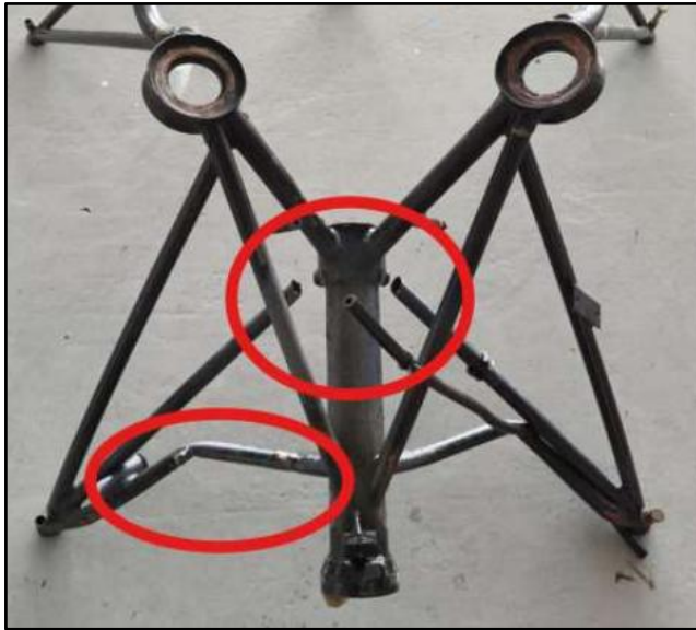
Figure 5: Both lower engine mount tubes bent inward as a result of the strong impact. Due to a hard impact, both centre engine mount tubes cracked, had completely broken off at the welding spot.
