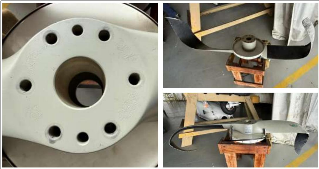
Figure 3: Both blade tips twisted inward, causing serious damage to blade and hub
