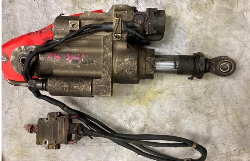
Figure 21. Left roll control actuator.
