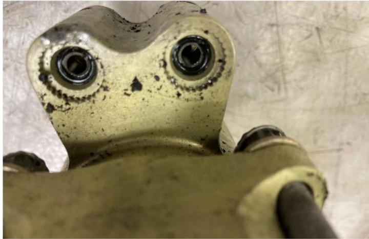
Figure 13. Right pull down actuator showing hydraulic ports.
