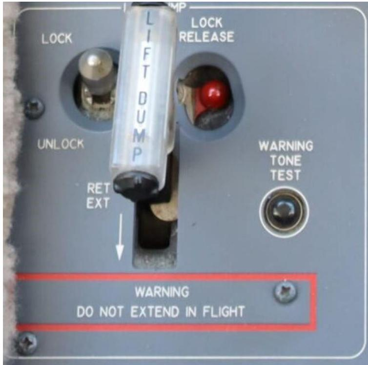
Figure 2. Exemplar lift dump panel. (Courtesy of Textron Aviation).
