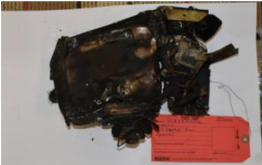
Figure 41. Lift Dump Panel recovered from the wreckage.
