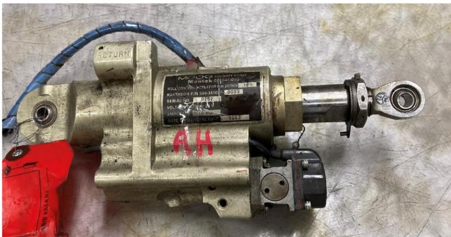
Figure 6. Right roll control actuator.
