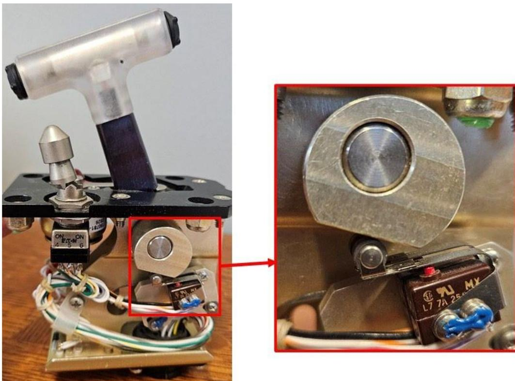
Figure 5. Exemplar lift dump handle – showing the left side in the RET (retract) position including a zoomed in view of the microswitch. (Courtesy of Textron Aviation).
