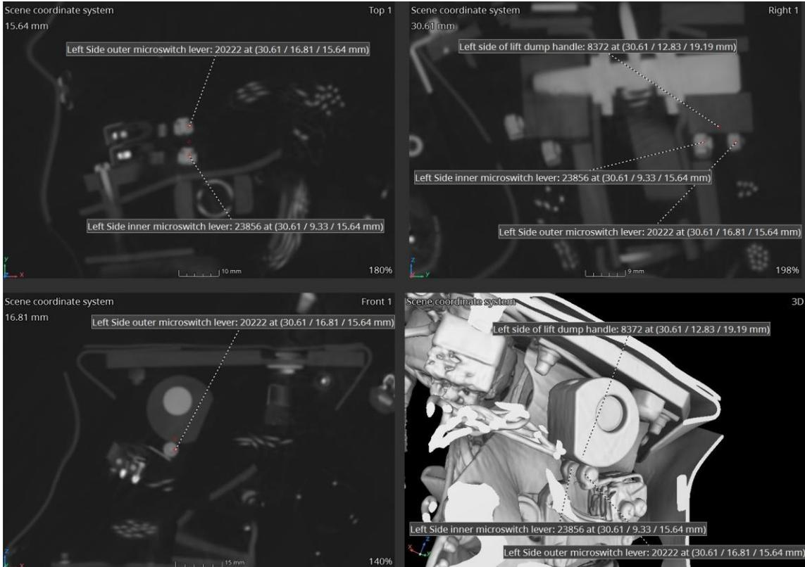
Figure 13. Image of lift dump panel - showing the left side.
