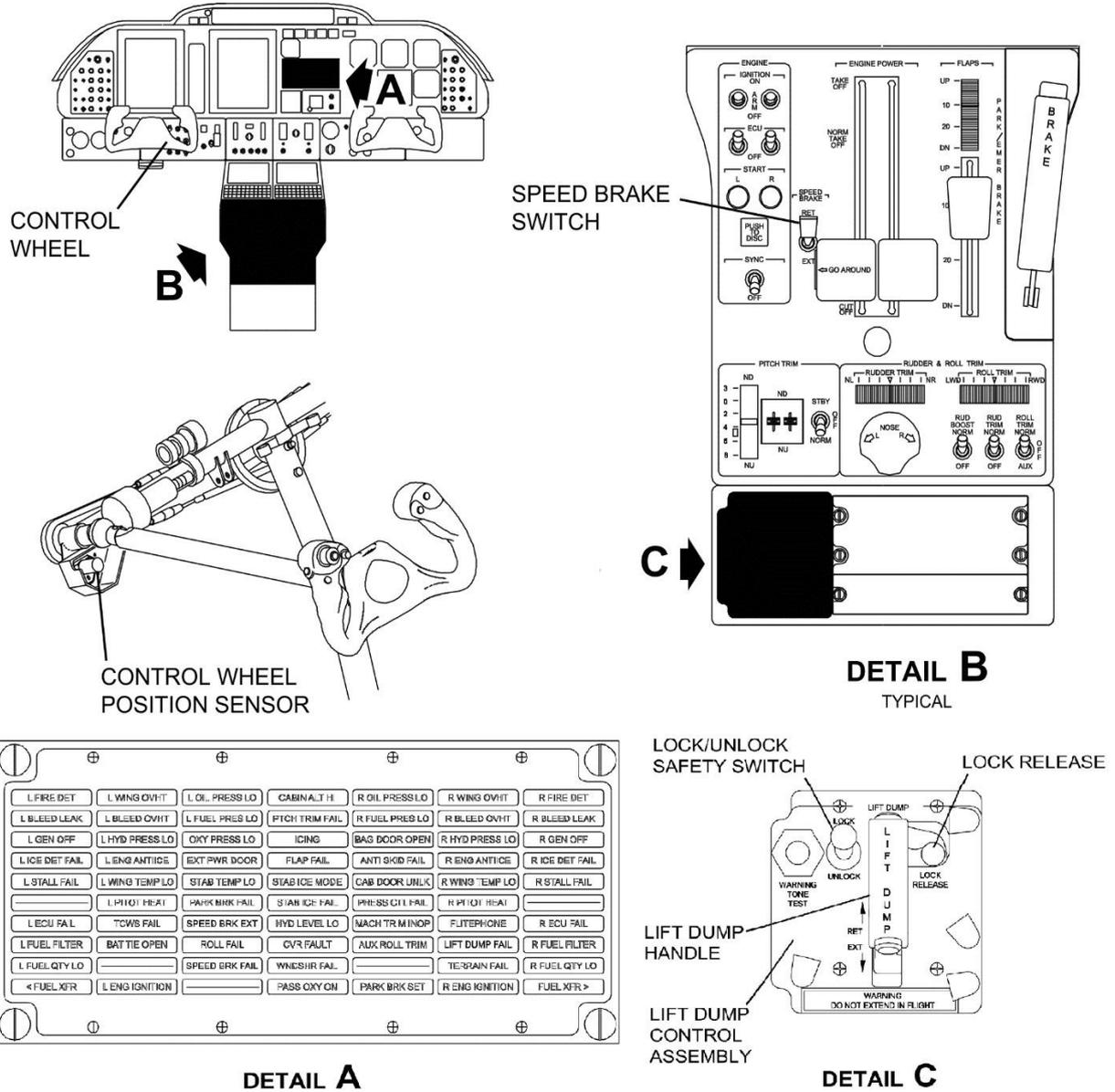
Figure 1. Spoiler System – Cockpit Components. (Courtesy of Textron Aviation).
