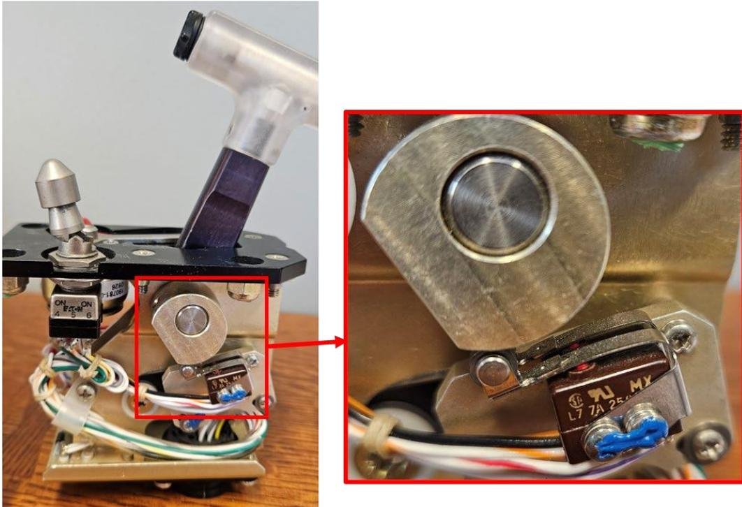
Figure 6. Exemplar lift dump handle – showing the left side in the EXT (extend) position including a zoomed in view of the microswitch. (Courtesy of Textron Aviation).
