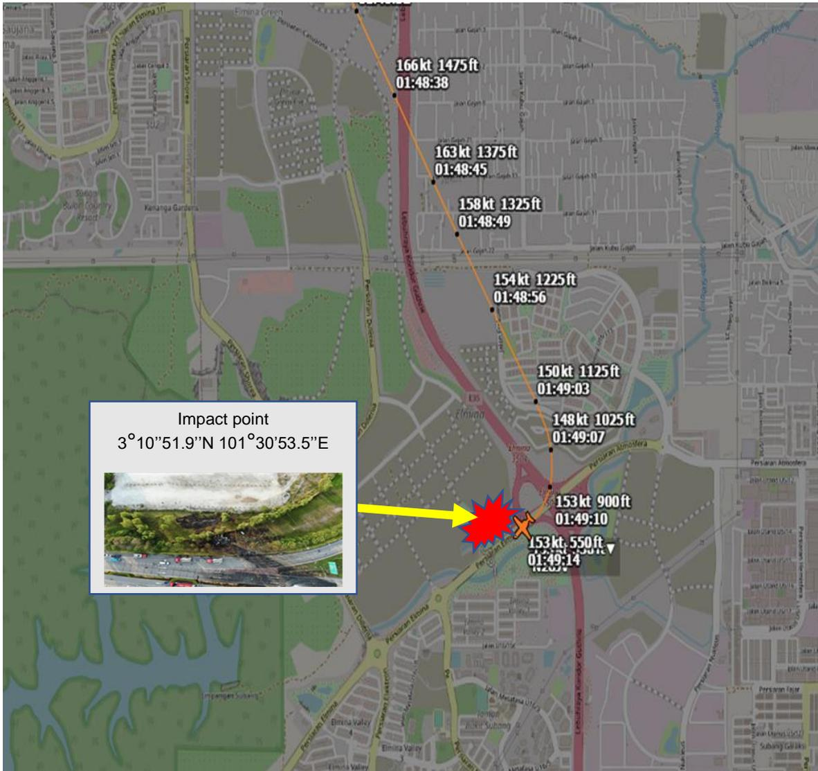
Figure 2. N28JV Impact Point<sup>2</sup>.
