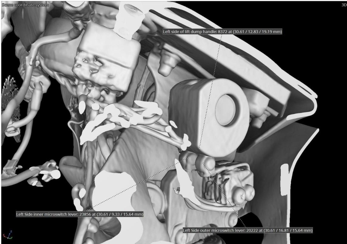
Figure 14. Image of lift dump panel - showing the left side of 3D image.
