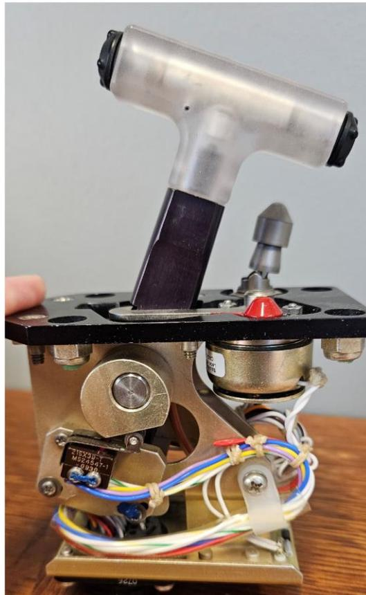
Figure 3. Exemplar lift dump handle – showing the right side in the RET (retract) position. (Courtesy of Textron Aviation).
