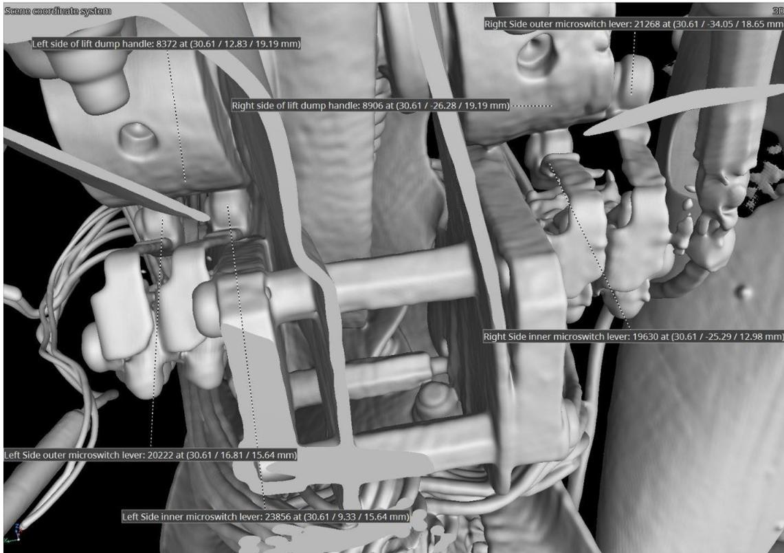
Figure 16. Image of lift dump panel – view looking forward.
