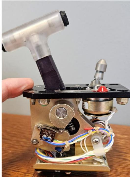
Figure 4. Exemplar lift dump handle – showing the right side in the EXT (extend) position. (Courtesy of Textron Aviation).
