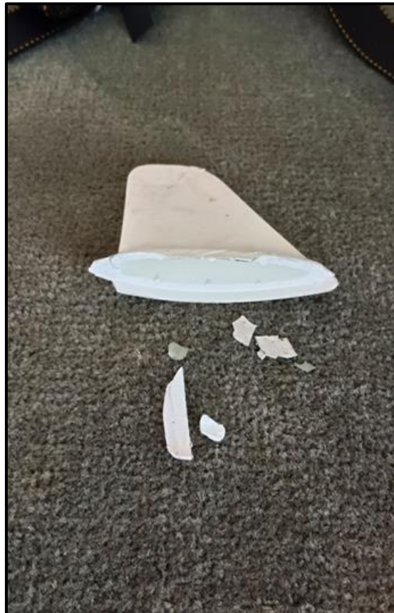
Figure 4: DME Antenna broken
