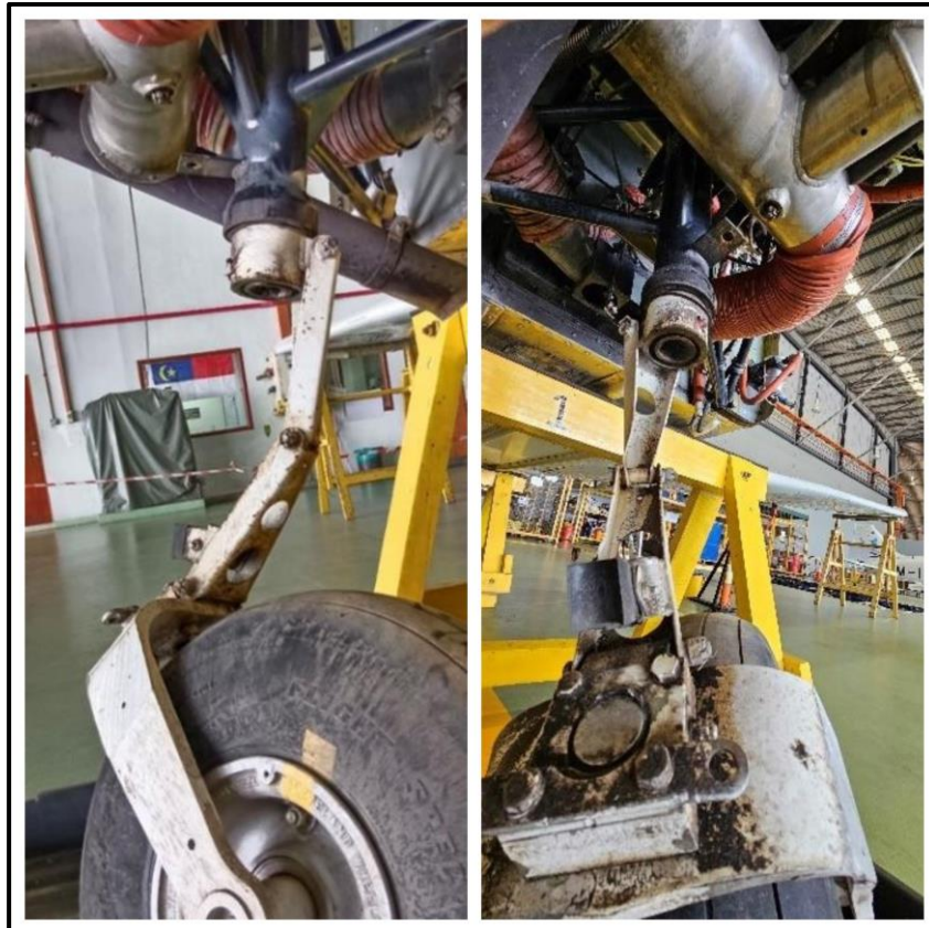
Figure 2: Broken nose landing gear (NLG)
