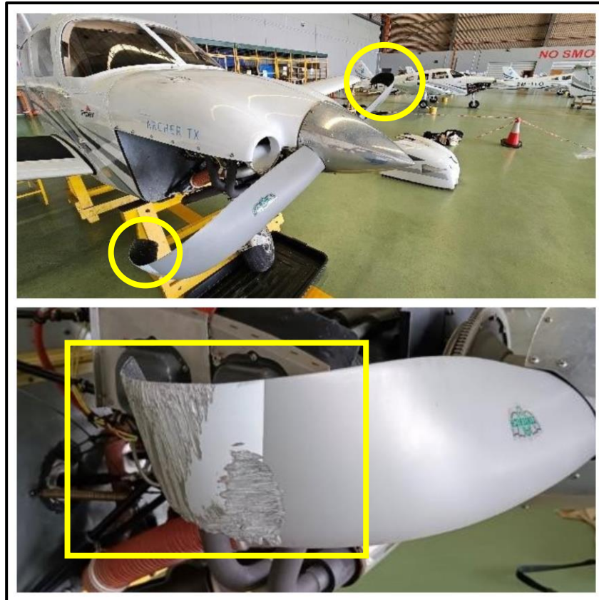
Figure 1: Bent and scratches on both sides of the propeller
