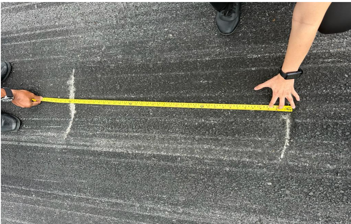
Figure 11: Scratched marking from the propeller strike during the first attempt to land
