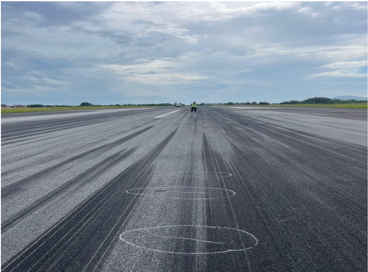
Figure 12: Scratched marking from the propeller strike during the second attempt to land
