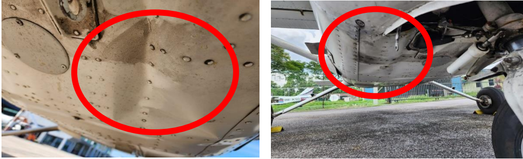
Figure 4: Lower Fuselage Skin dented
