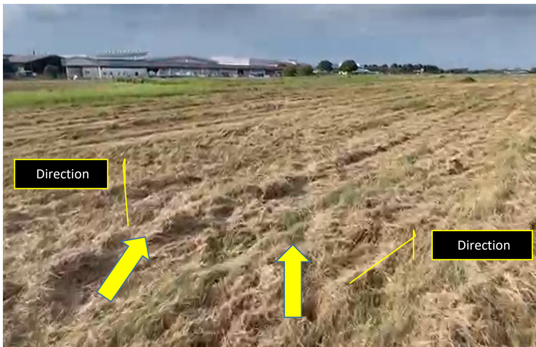
Figure 12: Aircraft tire track marks were observed exiting the runway towards the crash site.
