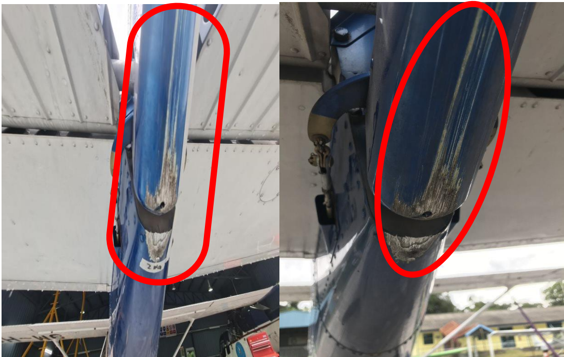
Figure 6: Rudder Lower tip found scratches
