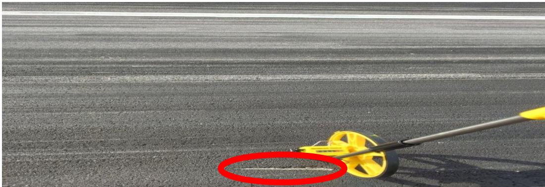
Figure 11: Scratched marking from the rudder lower tip on the runway during the hard landing.
