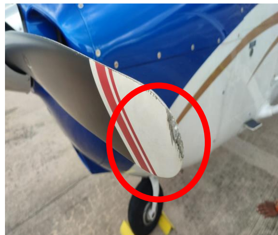
Figure 2: All Propeller blades bent inwards at the blade tips.
