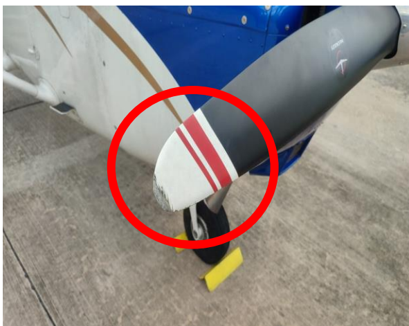
Figure 2: All Propeller blades bent inwards at the blade tips.
