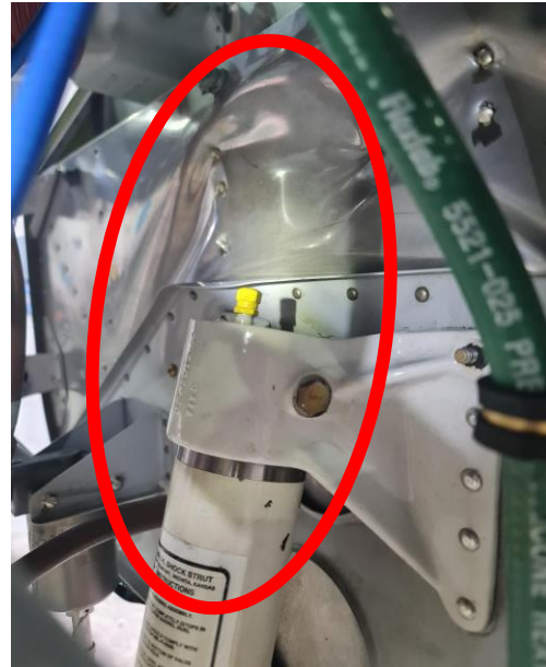
Figure 3: Nose landing gear. Damaged on riveted joints.
