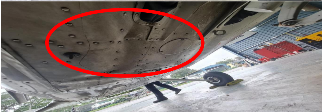
Figure 4: Below fuselage. Found deep scratches.
