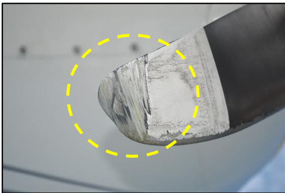
Figures 2 and 3: Scratches on both propeller tips
