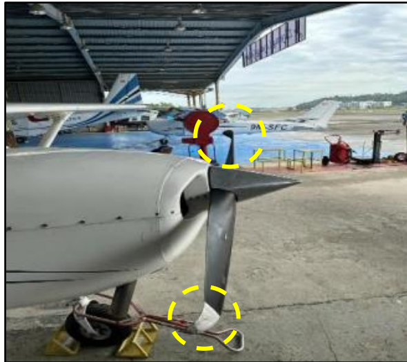
Figure 1: Bent on both sides white area of the propeller
