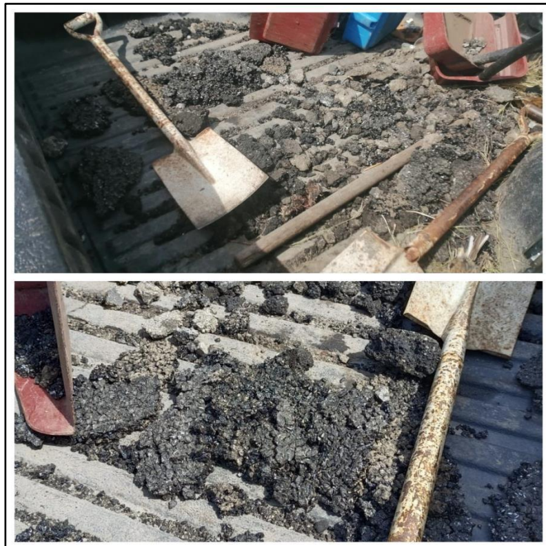
Figure 8: Debris collected after a few days of collection behind the MASB vehicle used for the runway inspection.
